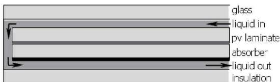
**Figure 1:** Schematic overview of the dual flow concept.
