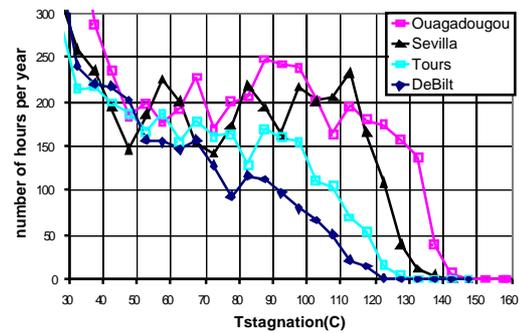
**Figure 9:** Stagnation temperature frequency plot (in intervals of 5 C) for different locations, as calculated with the dynamical model using Meteonorm data.
