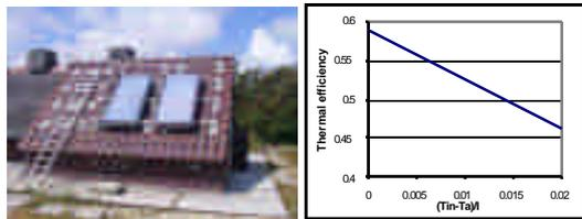
**Figure 2:** PVT collectors and measured thermal efficiency curve of the PVT collector
