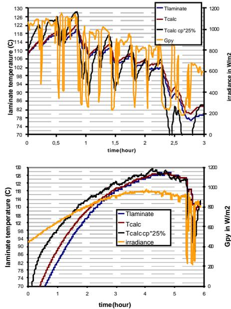
**Figure 5:** Comparison of calculated and measured laminate temperatures together with ambient conditions on a cloudy day (upper figure) and a clear day (lower figure).
