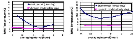
**Figure 7:** The effect of the averaging interval on the RMS value of the difference between the measured and the calculated stagnation temperature, using a steady state model or a dynamic model.
