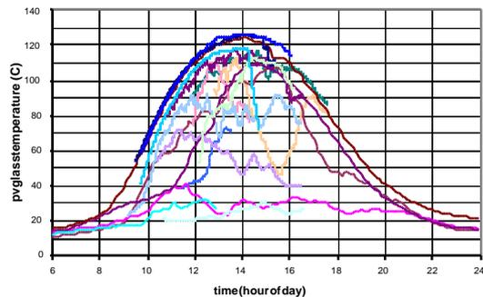
**Figure 3:** Measured stagnation temperature over various days, May-August 2002 ( $T_a$  14 to 30 °C,  $v_{wind}$  1 to 8 m/s)
