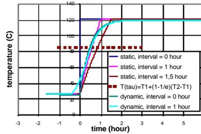
**Figure 6** The effect of the averaging interval over a step function as compared to the dynamic model
