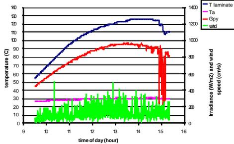
**Figure 4:** Stagnation temperature and ambient conditions measured on 29-7-2002.
