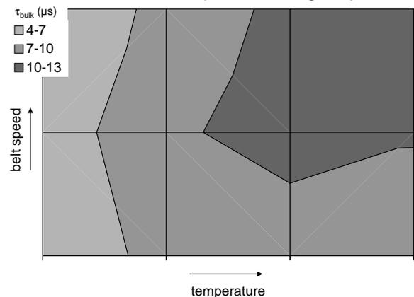
Figure 6: Contour plot of the minority carrier bulk lifetime as a function of belt speed and firing temperature.
