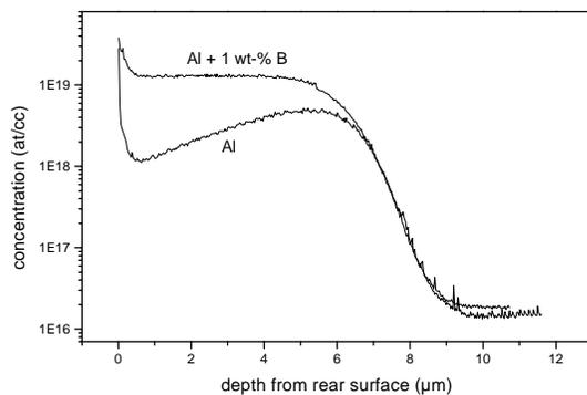
Figure 4: Dopant concentration of a BSF made with and without a boron addition to the Al-paste. Measured using ECV.
