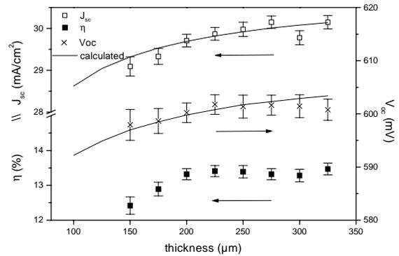
Figure 2:  $J_{\text{sc}}$  and  $V_{\text{oc}}$  and  $\eta$  as a function of the wafer thickness. Error bars show 95% confidence limits. Solid curves are calculated with PC1D using the parameters given in Table 2 and  $S_{\text{front}} = 10^6$  cm/s,  $L_{\text{BSF}} = 0.4 \mu\text{m}$ , and  $L_{\text{bulk}} = 300 \mu\text{m}$ . N.B.  $L_{\text{BSF}} = 0.4$  corresponds to  $S_{\text{eff.back}} = 4200$  cm/s.
