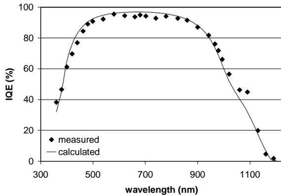
Figure 1: IQE data for 325  $\mu\text{m}$  wafer. Solid curves are calculated using PC1D: best fits are obtained for  $L_{\text{bulk}} = 300 \mu\text{m}$ ;  $L_{\text{BSF}} = 0.4 \mu\text{m}$ ,  $S_{\text{front}} = 10^6$  cm/s
