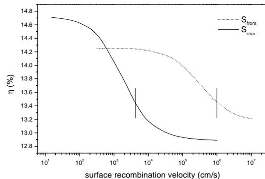
Figure 3: Effect of surface passivation on the efficiency of a 200  $\mu\text{m}$  thick wafer. The curves are calculated with PC1D using the parameters given in Table 2 and  $L_{\text{bulk}} = 300 \mu\text{m}$ ,  $S_{\text{front}} = 10^6$  cm/s (in calculating the dependence of  $S_{\text{rear}}$ ) and  $S_{\text{rear}} = 4200$  cm/s (in calculating the dependence of  $S_{\text{front}}$ ). The vertical markers indicate the experimental surface recombination velocities.
