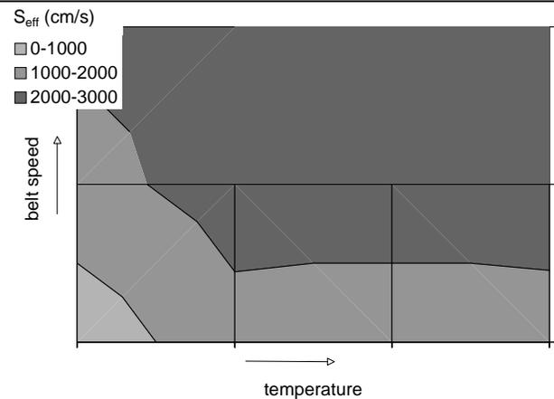
Figure 5: Contour plot of the effective rear surface recombination velocity of an Al-BSF as a function of belt speed and firing temperature.
