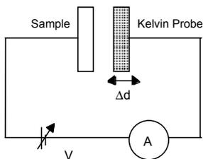
Fig. 2: Equivalent electronic circuit for KP-measurements
