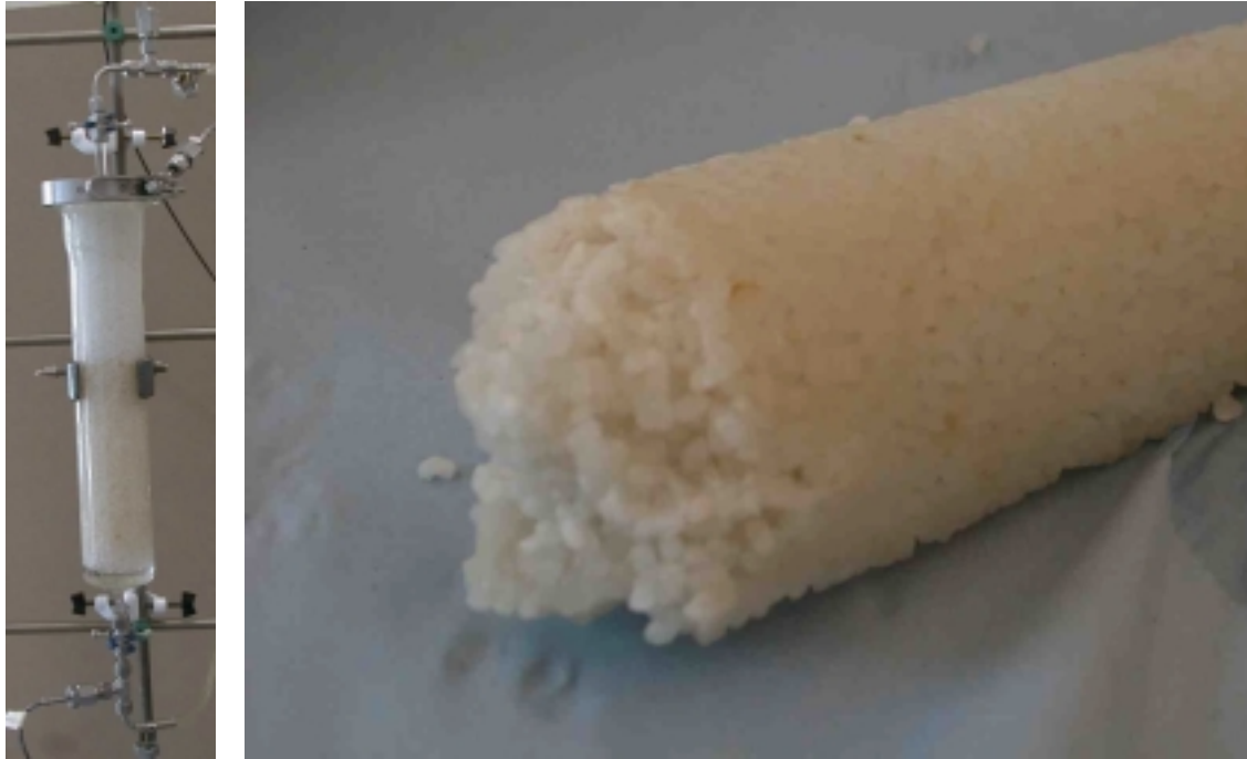
Figure 1.3 Test container and the porous structure of the paraffin grains
