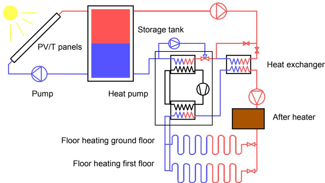
In days of high temperatures of the water in the storage tank (and heating demand), the heat from the storage tank will be transferred to the floorheating system with the help of the heat exchanger. In the days of low temperatures of the water in the storage tank (and heating demand), a heat pump will be used to transfer the heat of a low temperature from the storage tank to heat of a high temperature so that the heat can be used for the floorheating system of the house.
