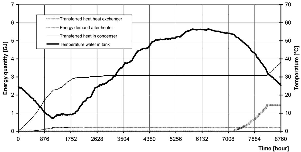
With this system, the thermal and electrical efficiencies are 28.2 and 2.5 %. The electrical efficiency is low because a part of the electrical energy will be used for driving the compressor of the heat pump. This part is not counted in the electrical efficiency. This system can supply 95.8 % of the total heating demand of the house.
