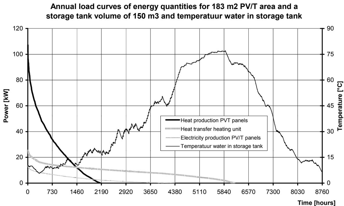
With this system, the thermal and electrical efficiencies are 27.0 and 6.9 %, with a solar fraction of 55.3 % of the ventilation air heating demand.
