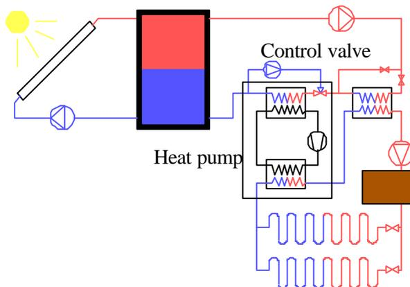
With the system without the heat pump, the after heater will be used if the temperature of the water in the storage tank is lower than the supply temperature of the floorheating system (=35 °C). By introducing a heat pump in the system, the heat of the water in the storage tank can be used in cases that the temperature of the water is lower than the supply temperature for the floorheating system.
