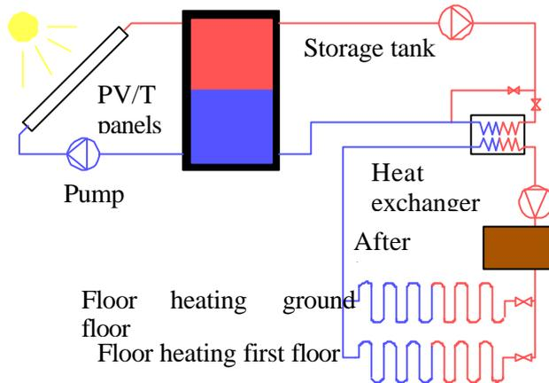
As well as using the PV/T panels for making domestic hot water and preheating the ventilation air, the panel can also be used for a low temperature heating system for a house. The problem is that a house has the largest heating demand during wintertime. The winter is the period with the minimum quantity of sunshine. This implies that you have to store the heat in the summertime so that you can use it in wintertime. This will be realized by using a big seasonal storage tank filled with water.
