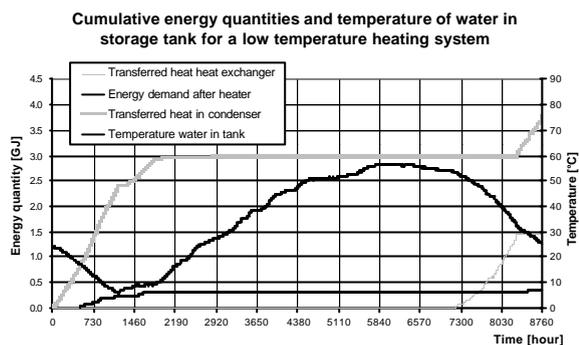
With this system, the thermal and electrical efficiencies are 28.0 and 2.7 %. This system can supply 95.8 % of the total heat demand of the house.
