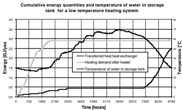
With this system, the thermal and electrical efficiencies are 6.7 and 7.6 %. This system can supply 45.4 % of the total heating demand of the house.
