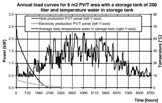
With this system, the thermal and electrical efficiencies are 22.1 and 6.8 %, with a solar fraction of 50.5 % of the total heating demand for hot water.
