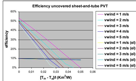
Figure 5: Thermal and electrical efficiency for the uncovered sheet-and-tube collector.
