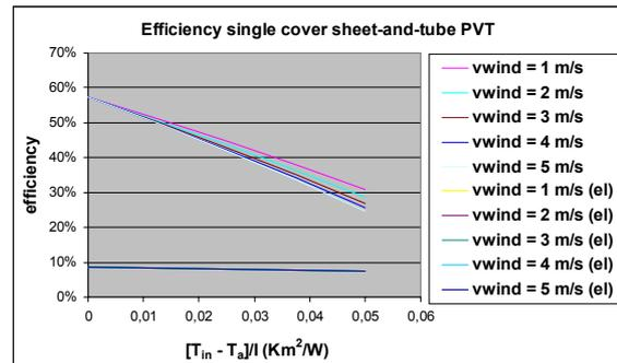
Figure 6: Thermal and electrical efficiency for the covered sheet-and-tube PV thermal concept.
