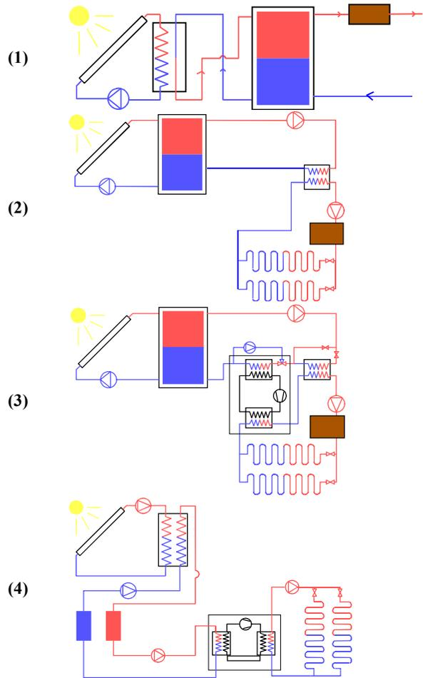
Figure 9: System concepts. Top to bottom: (1) domestic hot water, (2) domestic heating, (3) domestic heating with heat pump, (4) domestic heating with heat pump and aquifer.
