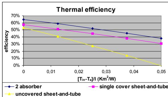
Figure 3: Thermal efficiency curves
