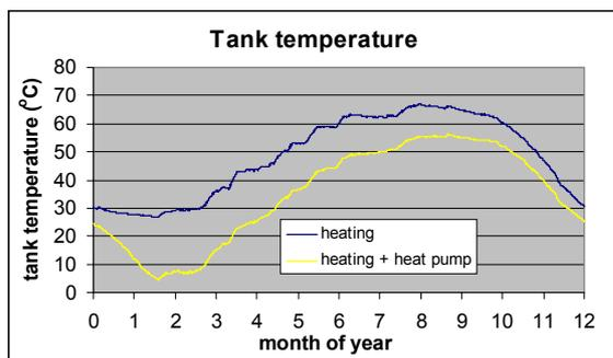
Figure 15: The temperature in the 20 m<sup>3</sup> storage tank for the case with and without heat pump (for the calculation with covered sheet-and-tube collector).
