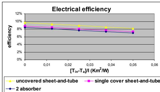
Figure 4: Electrical efficiency curves
