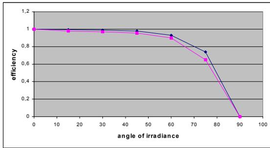
Figure 7: Effect of angle on transmission of irradiance.
