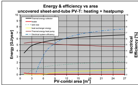
**Figure 12: The size optimisation for domestic heating system with heat pump in combination with the uncovered sheet-and-tube PVT concept.**
