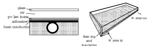
Figure 1: Sheet-and-tube PV thermal
