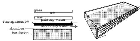
Figure 2: Two absorber channel PV thermal
