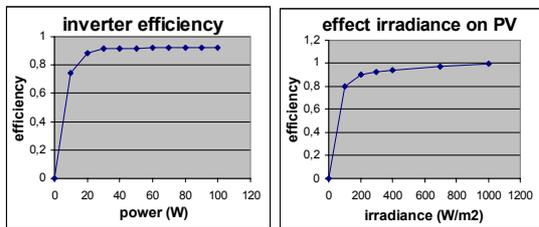
Figure 8: Left: Effect of low power on inverter efficiency. Right: Effect of low irradiance on PV efficiency.
