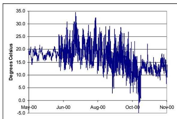
Figure 6. Temperature at the top of the battery box for system 9 over the period May to November 2000. Abrupt changes in the daily fluctuations are probably due to moving the system to a tent during the summer months.
