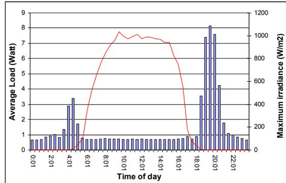
Figure 3. Maximum irradiance and average load in May 2000 for system 5. Compared to figure 2, the irradiance curve is much broader near the top.
