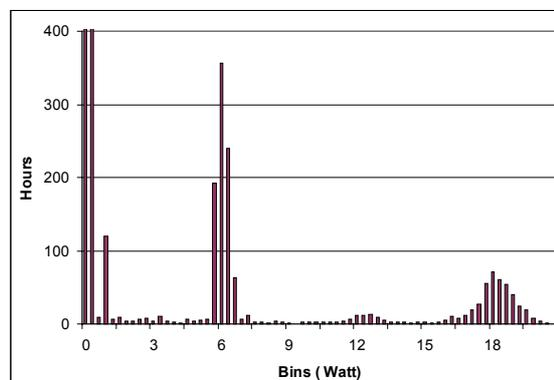
Figure 8 Load frequency distribution for system 7, showing the number of hours over the period June to November 2000 with a load within a range of 0.3 Watt bins.
