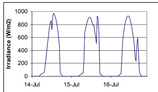
Figure 4. Irradiance graph for three consecutive days in 2000 for system 5. All three days show a distribution with two peaks, most probably caused by redirecting the module once a day. This explains the broad curve of figure 3.
