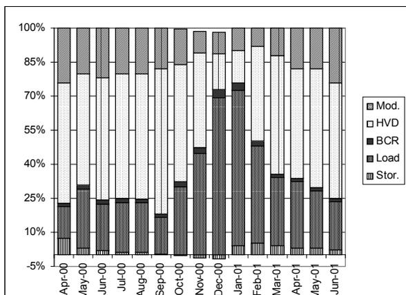
Figure 10. Energy balance of system 9 over the period April 2000 to June 2001. As a percentage of the reference yield the contribution is given of (from top to bottom): a) module losses, b) HVD losses, c) losses in the BCR d) net energy to load, e) net energy to storage.
