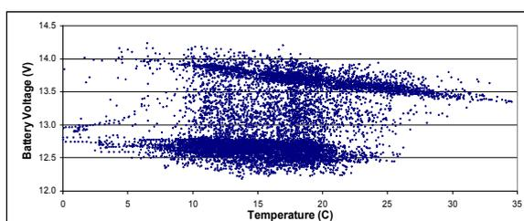
Figure 7. Ambient temperature versus battery voltage for system 9 from April to December 2000. The dots forming the inclined line at the top shows the temperature dependence of the high voltage disconnect setting.
