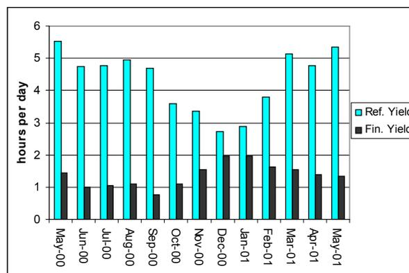
Figure 9. Reference yield and final yield (load) for system 9 for the period May 2000 to May 2001.
