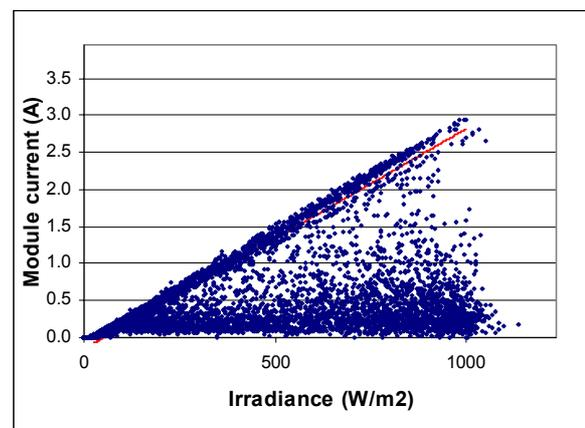
Figure 5. Irradiance versus module current for system 9. All the points below the straight line are supposed to indicate high voltage disconnect.
