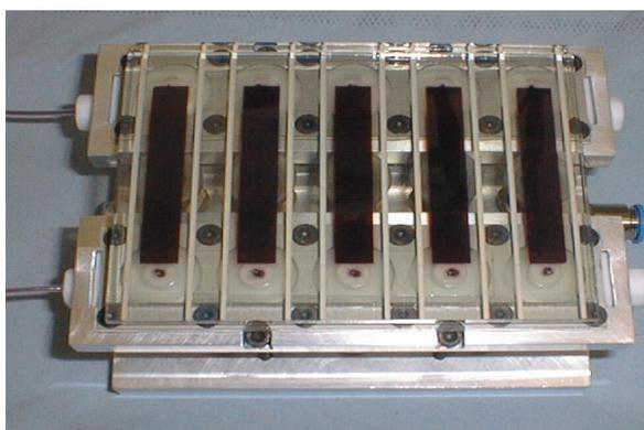
**Figure 1:** Processing of a master plate (75 mm x 100 mm) containing 5 individual dye sensitised test cells (active area 4 cm<sup>2</sup>). The coloration step, flushing of dye solution after sealing through holes on a filling unit, is shown.
