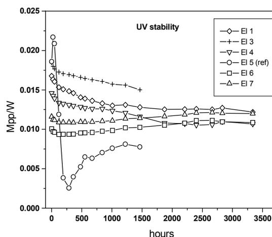
**Figure 2:** Stability data (maximum power point) of cells on masterplates after ageing with a UV-light tester (cell temperature 35 °C). Electrolyte no. 5 is the (unstable) reference without additive
