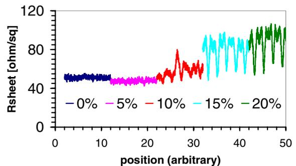
**Figure 4** Selectivity of emitter as a function of SiO<sub>2</sub> in barrier paste
