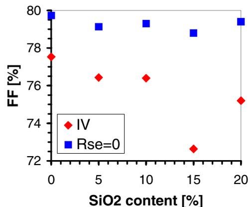
**Figure 7** Fill factors as determined by IV measurement and by Sinton measurement (series-resistanceless) as a function of SiO<sub>2</sub> content in barrier paste
