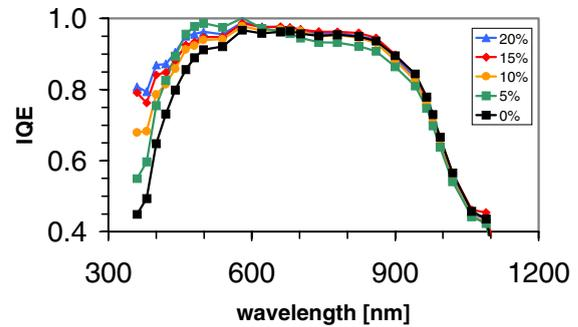
**Figure 9:** Internal quantum efficiency as a function of wavelength determined for 0% to 20% SiO<sub>2</sub> in barrier paste
