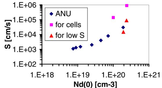
**Figure 13:** Surface recombination velocity as a function of emitter sheet resistance, for values determined in this study (for cells), ECN values determined for  $\text{SiN}_x$  (for low  $S$ , as it is optimised for surface passivation), and values from literature (ANU, Australian National University) also optimised for surface passivation [13]
