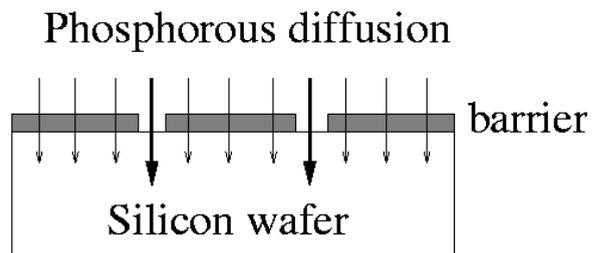
Figure 1 Principle of new selective emitter process.
