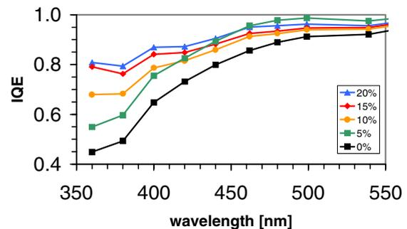
**Figure 10:** Detail of internal quantum efficiency as a function of wavelength determined for 0% to 20% SiO<sub>2</sub> in barrier paste
