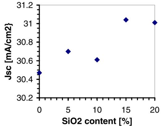
**Figure 5:** Short circuit current density as a function of SiO<sub>2</sub> content in barrier paste
