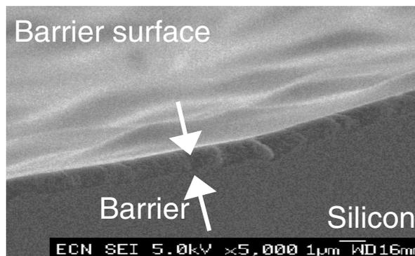
**Figure 2:** Scanning electron microscope photograph of a sintered SiO<sub>2</sub> layer deposited on a silicon wafer viewed in cross section; light material is the surface of the barrier layer
