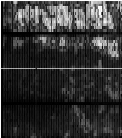
**Figure 9:** CoreScan of contact resistances measured locally on a cell with reduced fill factor (15% SiO<sub>2</sub> content), light spots indicate higher contact resistance
