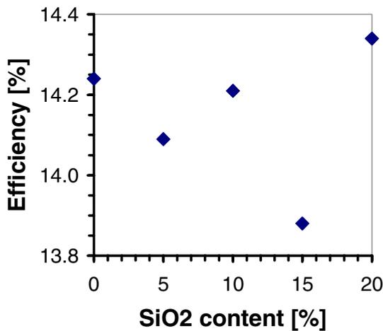
**Figure 8:** Efficiency as a function of SiO<sub>2</sub> content in barrier paste
