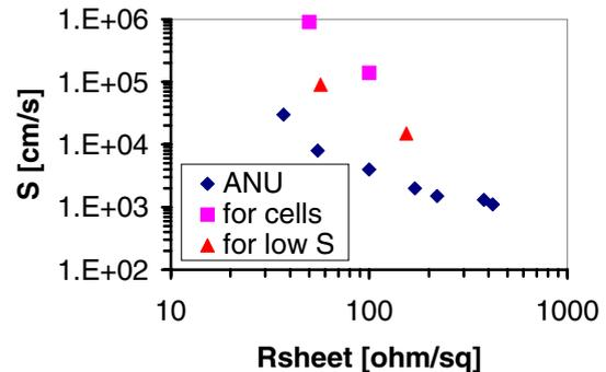
**Figure 12:** Surface recombination velocity as a function of emitter sheet resistance, for values determined in this study (for cells), ECN values determined for  $\text{SiN}_x$  (for low  $S$ , as it is optimised for surface passivation), and values from literature (ANU, Australian National University) also optimised for surface passivation [13]
