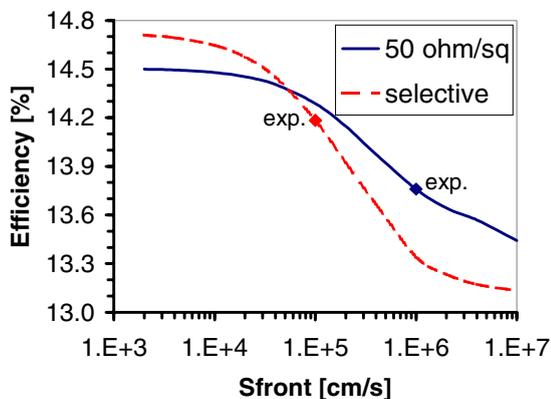
**Figure 11:** Calculated efficiency as a function of surface recombination velocity, for a homogeneous emitter profile (50 ohm/sq), and a selective emitter profile (20%  $\text{SiO}_2$  content), two points are indicated corresponding to  $S$  values fitted to experimental IQE values.
