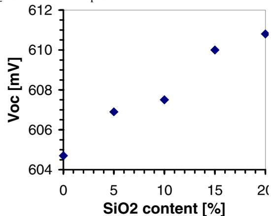
**Figure 6:** Open circuit voltage as a function of SiO<sub>2</sub> content in barrier paste
