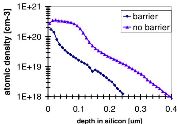
**Figure 3:** Stripping Hall measured doping profiles for samples with and without diffusion barrier.
