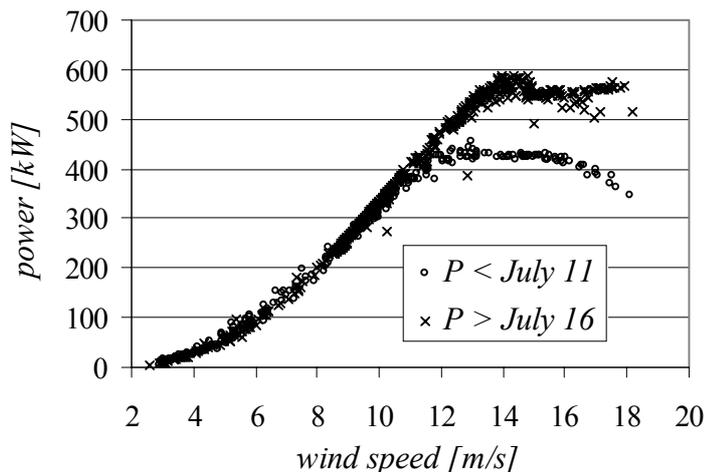
**figure 1** This figure shows an example of the power levels measured by Oak Creek Energy on a NEG Micon 700/44. The cause of this behaviour was unknown.
