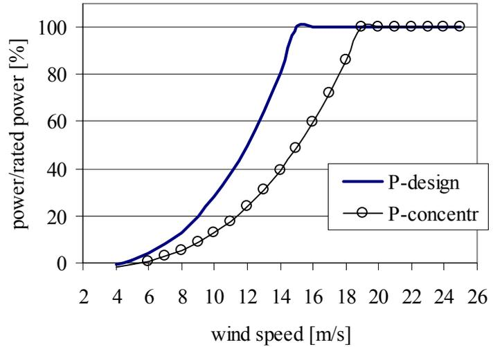
**figure 2** In the terrain concentration model the power is affected especially below rated power.
