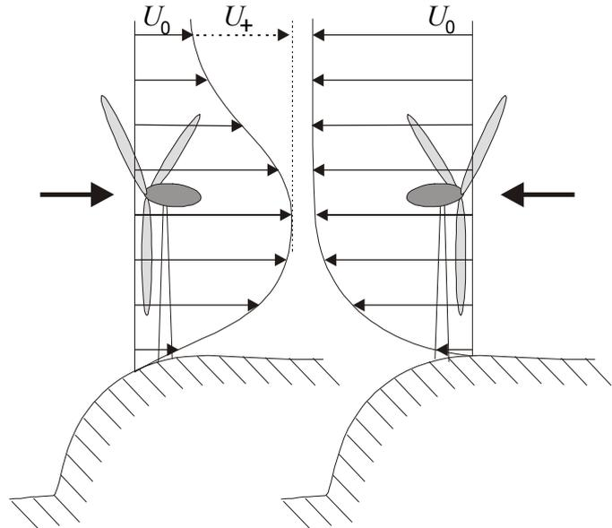
**figure 4** *The terrain concentration hypothesis. The wind speed measured on the nacelles of both turbines are equal, but the turbine on the left-hand side can extract less energy.*
