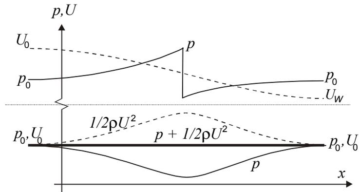
**figure 3** The lapse of pressure and speed for a wind turbine and a concentrator.
