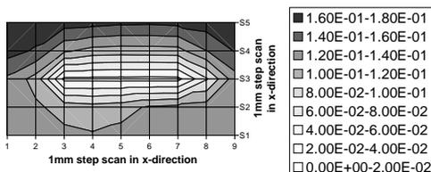
**Figure 6:** Voc mapping of a shunted (Ni)Al contact (legend: Voc inV)
