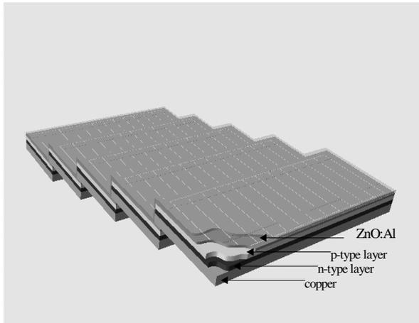
**Figure 6:** Roof-tile integrated CISCuT- module
