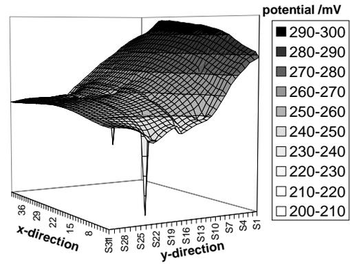
**Figure 3:** PRAMP mapping of a (9x9) mm<sup>2</sup> CISCuT cell (potential of 300 mV applied at the (NiCrCu)Sn contact)
