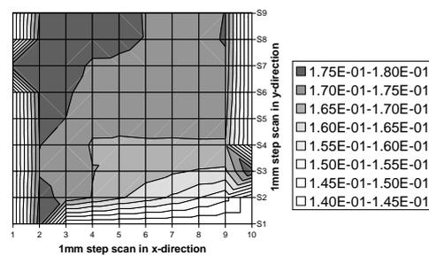
**Figure 4:** Voc mapping of a (9x9) mm<sup>2</sup> CISCuT cell at bias irradiation (legend: Voc in V)
