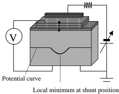
**Figure 2:** PRAMP principle tailored to the specific CISCuT cell configuration
