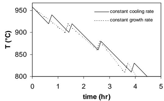
**Figure 3:** temperature profiles used in LPE deposition.
