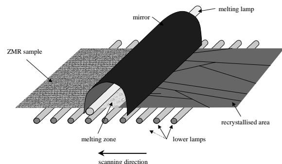
Figure 1: schematic drawing ZMR system
