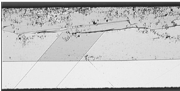
**Figure 2b:** fully recrystallised PS-Si coating on mc-Si.
