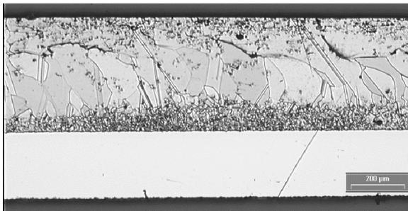
**Figure 2a:** partly recrystallised PS-Si coating on mc-Si.
