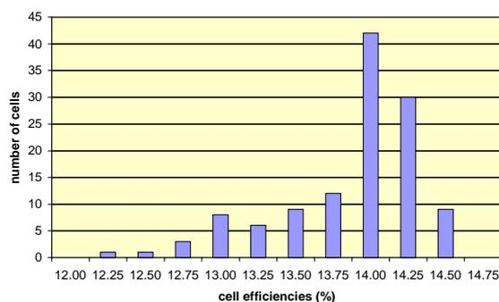
**Figure 3:** Histogram of mc-Si cell efficiencies for the 'firing through' process.
