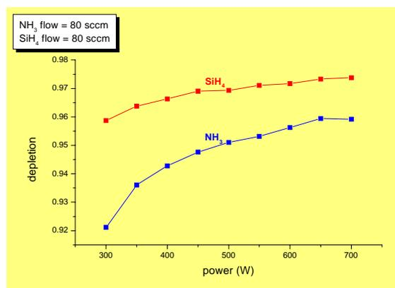
**Figure 5:** Depletion rates of SiH<sub>4</sub> and NH<sub>3</sub> during deposition of SiN.
