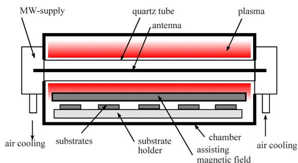
**Figure 2:** Schematic view of the plasma source.
