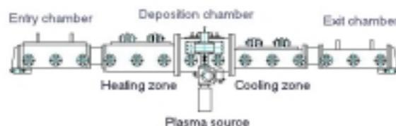
**Figure 1:** Side view of the pilot PECVD reactor.
