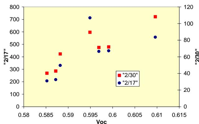
**Figure 6:**  $V_{oc}$  as a function of relative abundances of NH<sub>3</sub> (17 amu) SiH<sub>4</sub> (30 amu) versus hydrogen (2 amu) as measured by QMS.
