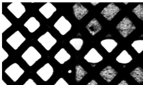
**Figure 1.** Back light photograph of emulsion type screen with part of the busbar (to the left) and finger (pointing to the right), showing the available open area for printing. Finger width in screen is 90  $\mu\text{m}$ .
