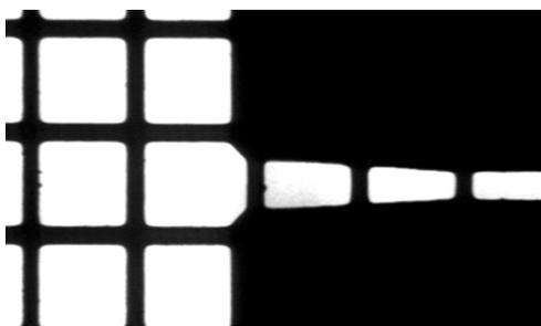
**Figure 2.** Photograph as in figure 1 of double layer stencil with part of the busbar (to the left) and finger (pointing to the right), showing the available open area for printing. Finger width in stencil 70  $\mu\text{m}$ .
