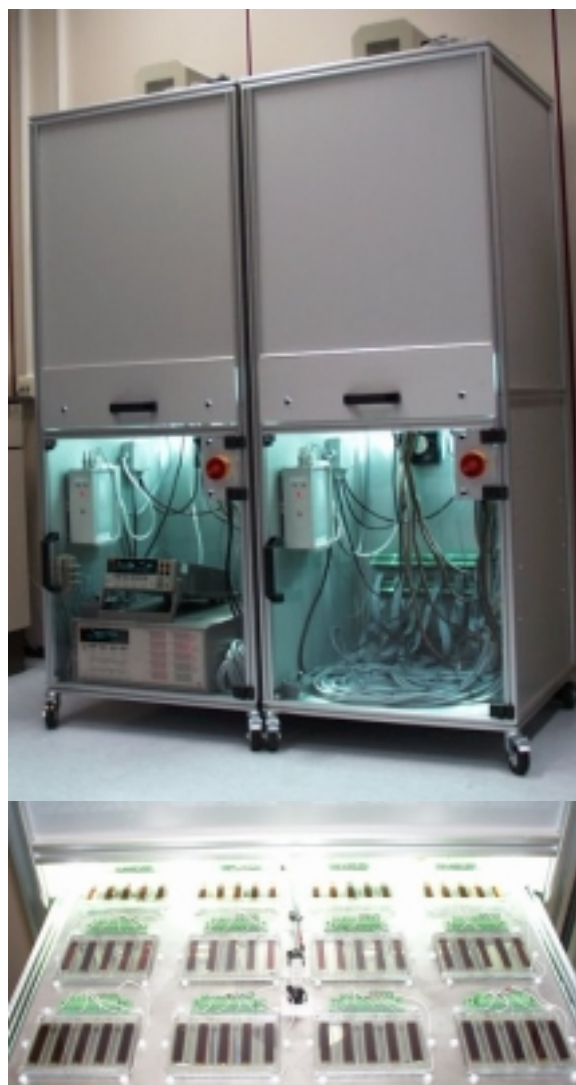
Figure 2: Photos of continuous illumination and characterisation sites for simultaneous light soaking experiments. At each site 16 master plates containing in total 80 test cells are operated under 1 sun equivalent sulphur lamp spectra. Masterplates in opened drawer are shown. Six such sites have been installed at the project partners.
