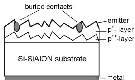
**Figure 7:** Schematic drawing of a thin film cell with Si infiltrated SiAlON substrate and LPE grown Si layers.
