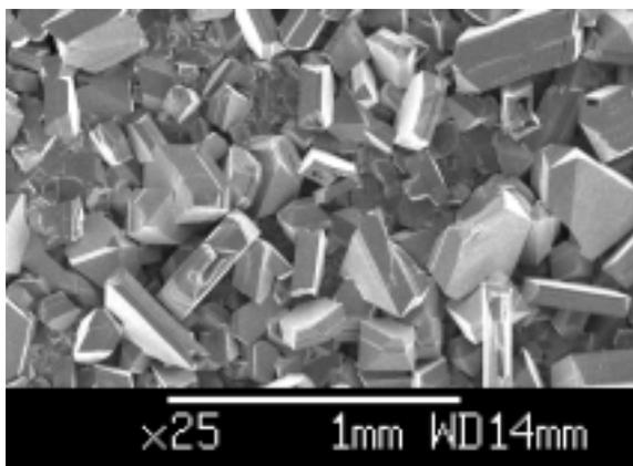
**Figure 5:** Si layer grown from Ga/Al solution on a Si infiltrated SiAlON substrate.
