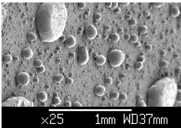
**Figure 2:** Si infiltrated SiAlON with 60% Si. The crystalline Si grains reach sizes up to 1 mm. The distance between grains has not decreased.
