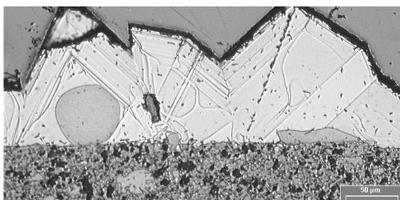
**Figure 6:** Etched cross-section of a Si layer grown from a Ga/Al solution on a Si infiltrated SiAlON substrate. Grey areas coming out of the substrate surface are the Si seed grains.
