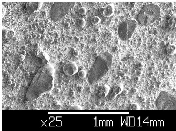
**Figure 1:** Si infiltrated SiAlON with 42% crystalline Si. The maximum size of the Si grains is 500  $\mu\text{m}$ .
