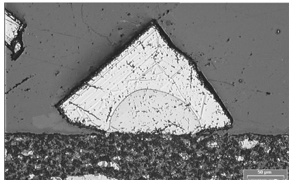
**Figure 3:** Semicircular Si grain from the substrate is epitaxially overgrown with Si during the LPE process. Etched cross-section.
