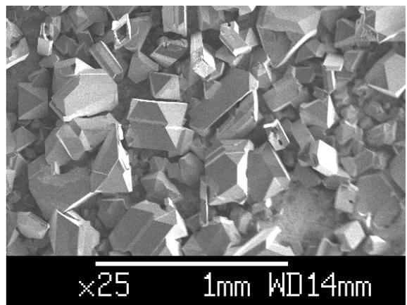
**Figure 4:** Si layer grown from Ga solution on a Si infiltrated SiAlON substrate. At some places the substrate is still uncovered.
