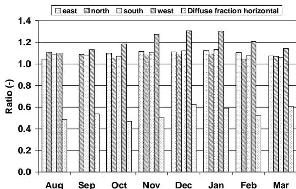
Figure 2 Ratio between the irradiance measured with the pyranometers and with the reference cells plus the diffuse fraction of the horizontal irradiance
