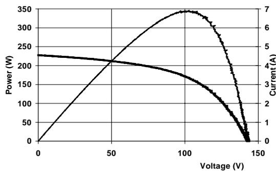
Figure 5 IV-curve at 42 °C and 820 W/m2
