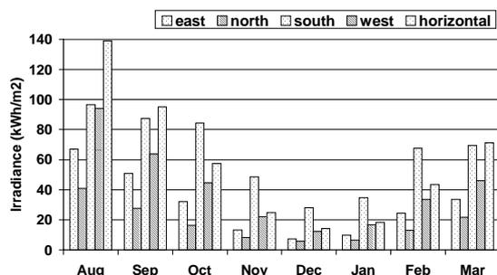
Figure 1 Monthly irradiation on the façades and on the roof (pyranometer data)
