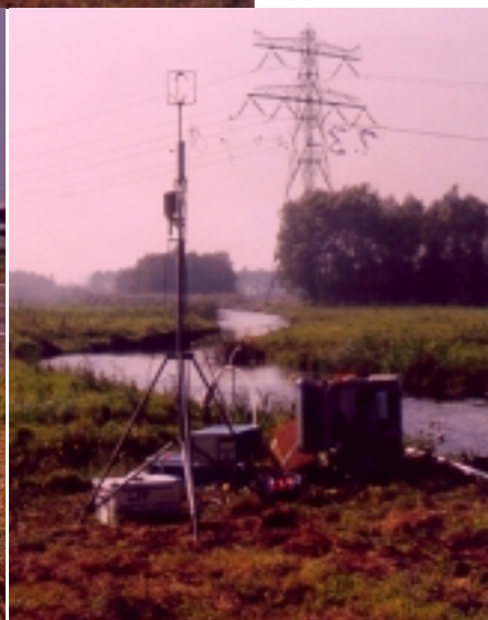
Figure 4.1 Photographs of the 23-9-98 A9 experiment. The above picture shows from left to right the SMPS/CPC combinations, the LAS-X and NO x monitors and the Sierra HVS impactor. The down-left picture shows the Sierra HVS, the PUF/Filter device and the Berner impactor. The down-right picture shows the meteo mast at 35 meter of the road with on top the Solent sonic anemometer, the NO x monitor and the data logging hardware.
