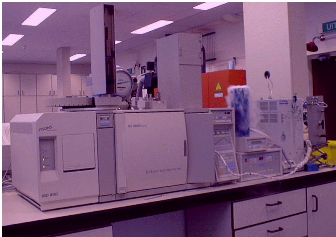
Figure 2.3 GC-MS system at the ECN laboratory
