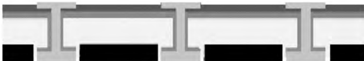
Figure 5.3: Illustration of a cross-section of the MWT cell. More details are given by Weeber et al. , Bultman et al. and de Jong et al. [58–60].
