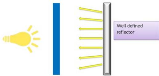
**Figure 4:** Schematic of Setup C with one light source illuminating the front of the module and a well-defined diffuse reflector behind the module at some distance.
