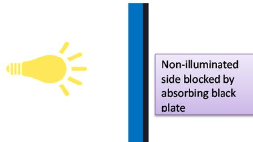
**Figure 3:** Schematic of Setup B with one light source and a non-reflecting black absorbing material is placed against the module on the non-illuminated side. Multiple measurements are necessary.
