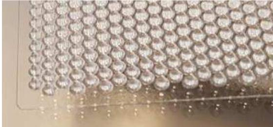
**Figure 2:** A close-up photograph of TOWA's structured AR coating on a solar glass substrate.
