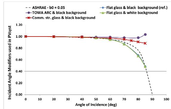
**Figure 4:** Measured Incident Angle Modifiers (IAMs) for a fixed azimuth, compared to the standard ASHRAE –  $b_0=0.05$  used in annual yield simulations; also included is a previously measured IAM for a commercial structured glass.
