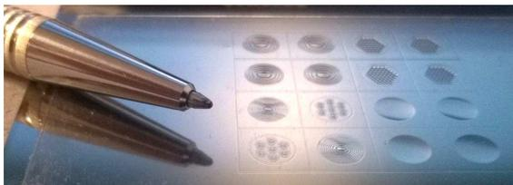
**Figure 1:** Examples of structures that can be produced using TOWA's high-pressure molding technology.
