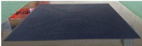
**Figure 3:** Single-cell laminate lay-outs manufactured and tested (top) and photograph of an IBC module having black rear encapsulant and glass coated with TOWA's AR coating (bottom).
