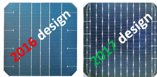
Figure 5. Mercury IBC former metallisation grid design with 31 contact pads (2016 design, left picture) and current metallisation grid design with 81 contact pads (2017 design, right picture) as processed at Yingli
