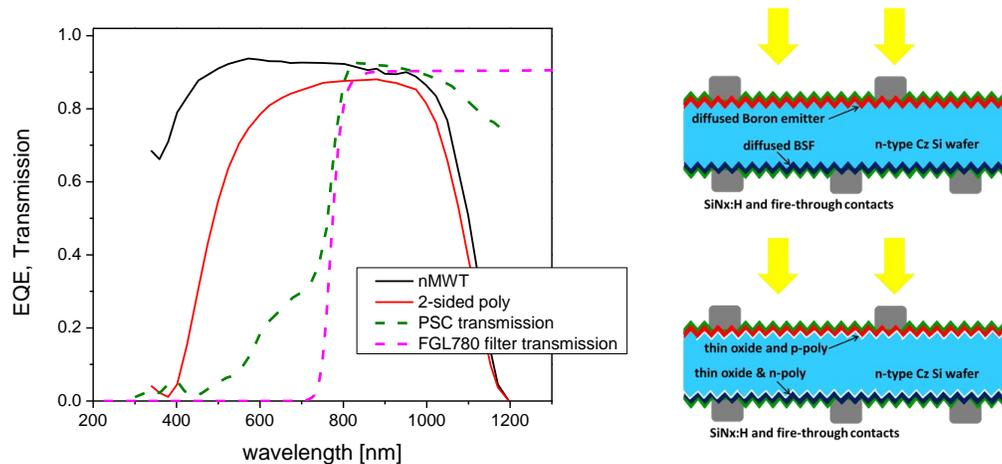
Fig. 2. Left: EQE of diffused and poly cells compared. Transmission of the PSC stack and longpass filter compared. Right: schematic cross section of the two cell types.
