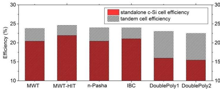
Fig. 3. Tandems based on different cSi bottom cells evaluated.
