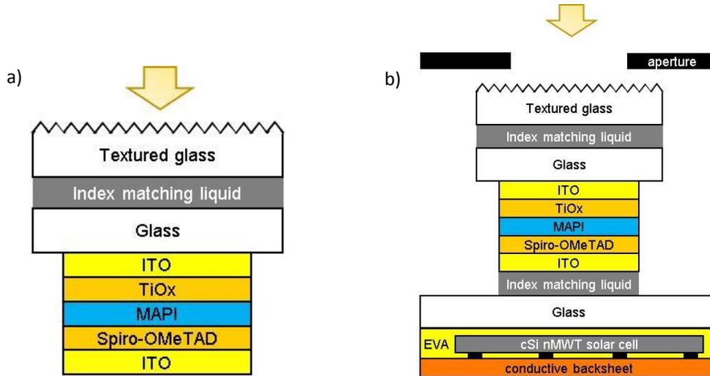
Fig. 1. a) Top cell configuration for single junction PSC measurement. b) Tandem configuration for measurement of the filtered  $J_{sc}$  of a small nMWT bottom cell. Aperture size  $25 \times 25 \text{ mm}^2$ .
