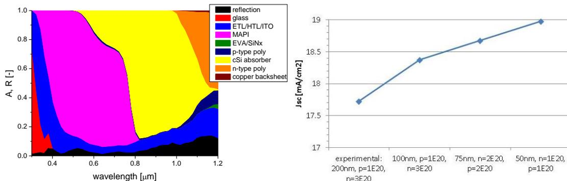
Fig. 4 .Left: optical model of the tandem based on the 2-sided poly FT cell. Right: illustration of the benefit of thinner and lower doped poly layers.
