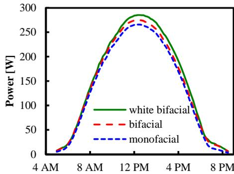
**Figure 8:** Example of the daily transient of the power output of the three modules on a sunny day.
