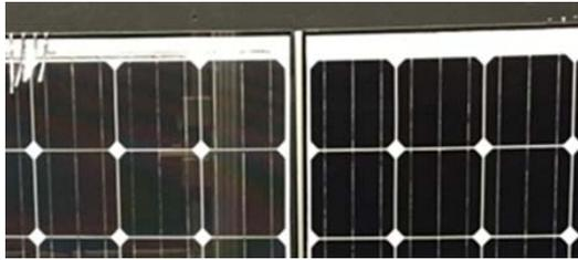
**Figure 1:** Close up photograph of the rear (left) and front (right) view of the white bifacial, double glass module. The white area between the cells and around the aperture area are well visible.
