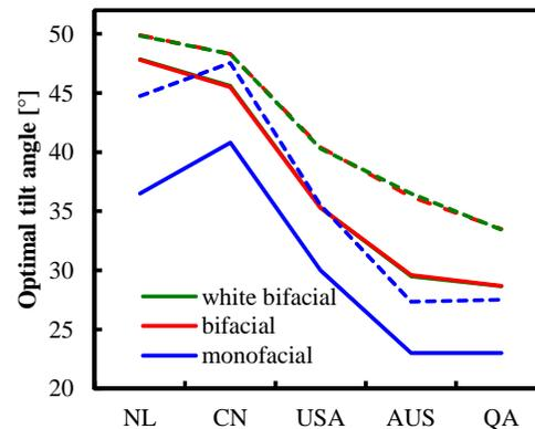
**Figure 7:** Optimal tilt angle for each combination of location, module type and albedo. Colours and dashes same as in Figure 6.
