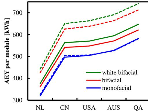
**Figure 6:** Modelled annual energy yield for the three different module types at five locations. Solid (dashed lines) are simulated with an albedo of 0.2 (0.5). Same colour represents same module type. Details of the locations are given in Table 2.
