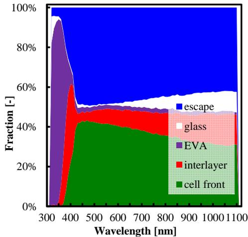
**Figure 4:** Ray tracing results for the white bifacial module for light incident on the intercell area.
