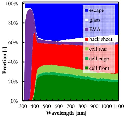
**Figure 3:** Ray tracing results for the monofacial module for light incident on the intercell area.
