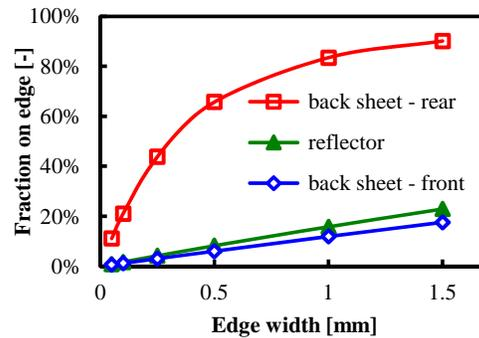
**Figure 5:** Fraction of the light incident on the edge of the front/rear side of the solar cell, as function of the edge width.
