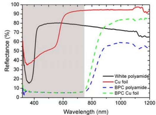
**Figure 3:** Reflectance data of the standard and BPC polyamide and Cu foils used in this study.
