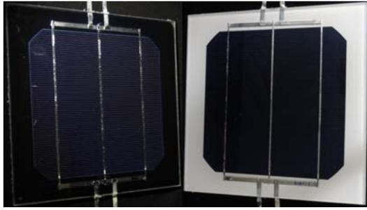
**Figure 2:** Images of single-cell laminates prepared with either white polyamide or black-powder coated polyamide.
