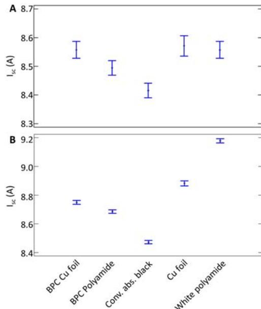
**Figure 4:**  $I_{sc}$  values recorded for the single cell laminates in case A) only the cell area and B) the full laminate is illuminated. In the latter case the illuminated area includes a 22 mm wide area around the cell where the backsheet is exposed to the incident light (see also Figure 2)
