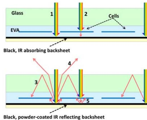
**Figure 1:** Illustration of the improved module light management in case of a black, IR reflecting backsheet. 1) Incident radiation absorbed by backsheet, 2) Transmitted (IR) radiation absorbed by backsheet, 3) IR part of incident radiation reflected and trapped at front, 4) As 3) but within escape cone, 5) Transmitted radiation reflected and re-entering cell through rear.
