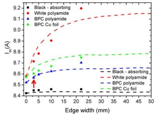
**Figure 5:**  $I_{sc}$  as function of the exposed edge width around the cell for different backsheets studied. The dashed lines are the result of a ray-tracing analysis using a simple model (for details see text).
