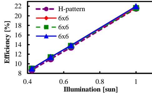
**Figure 4:** Efficiency as a function of the illumination level for H-pattern SHJ and 6x6 MWT-SHJ solar cells
