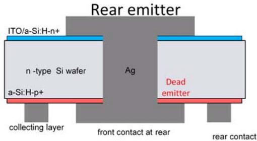
**Figure 1:** Schematic structure of a rear emitter MWT-SHJ solar cell. The collecting layer represents both the IWO:H and Ag rear contact
