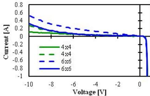
**Figure 3:** Reverse characteristics of MWT-SHJ solar cells with Ag screen printing for both 4x4 and 6x6 vias configuration
