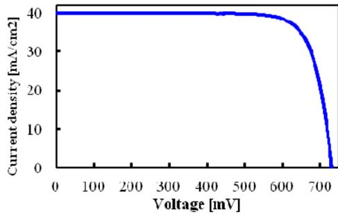
**Figure 2:** IV curve of the best MWT-SHJ solar cell with copper plating front side metallisation
