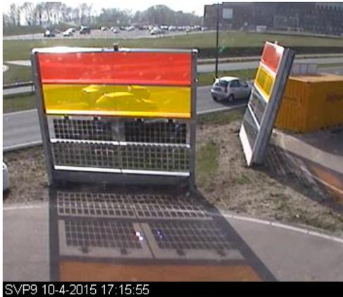
**Figure 3:** Photograph depicting the test setup of the two modular noise barriers
