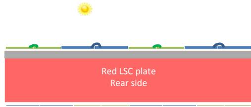
**Figure 9:** Schematic of the East/West oriented LSC in the morning looking from the East. The supporting construction induces a shadow (grey bar) along the top of the rear side, thereby affecting the output of the top cells
