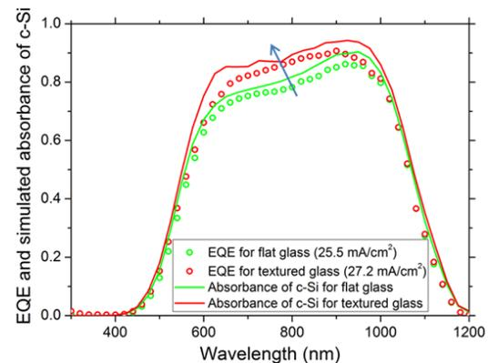
**Figure 5:** EQE of the c-Si bottom cell of a hybrid tandem, for which the front glass was flat (green) or coated with an AR texture (red)
