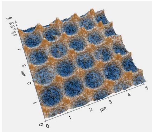
**Figure 6:** 2D periodic texture imprinted in a UV curable lacquer, after annealing at 550 °C. The  $R_{pv}$  is about 80 nm; i.e. about 50% of the  $R_{pv}$  of the master.
