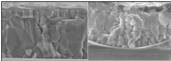
**Figure 7:** SEM cross section of CIGS solar cells on flat surface (left) and textured surface (right).
