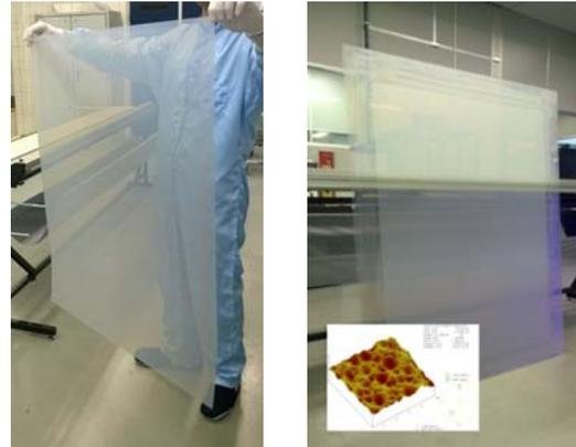
**Figure 8:** Large area shim (left) and imprint of a replica of sputtered-etched AZO (right)
