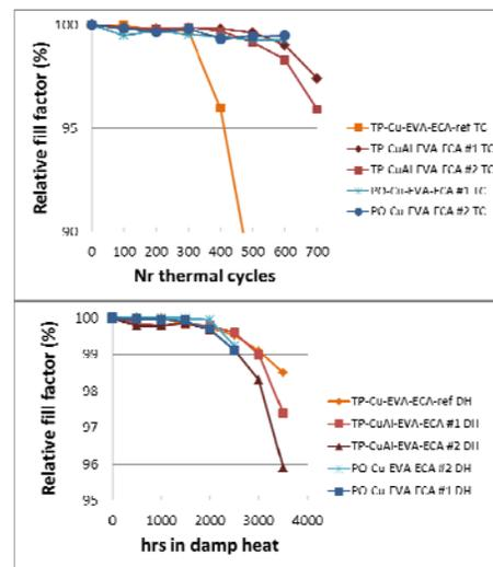
**Figure 3.** Effect of TC and DH exposure on the relative FF of p-MWT modules. main module components are indicated in the legend.
