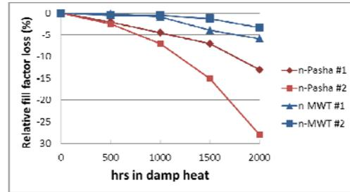
**Figure 5.** Effect of DH exposure on FF loss for frameless single-cell n-Pasha (tabbed cell) and n-MWT modules. Both types of modules were made with EVA.
