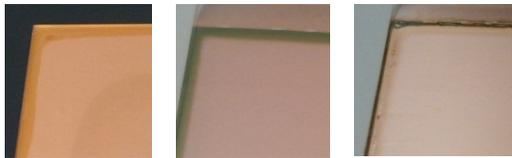
**Figure 4.** Visual appearance of glass-encapsulant-TP-Cu laminates after DH1500 test. Left: EVA; center: thermoplastic POE; right: thermosetting POE.
