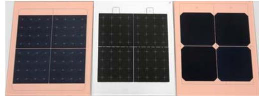
**Figure 2.** Photographs of some back-contact modules manufactured and tested at ECN for this study. Left: p-MWT module with TP-Cu foil. Middle: p-MWT module with TP-Al(Cu) foil. Right: IBC Mercury module.
