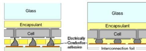
**Figure 1.** Cross section of a foil-based back-contact module before and after lamination.
