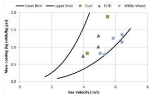
Figure 5: Mass loading of transport gas for lean-phase transport.
