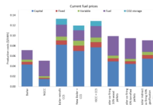
**Figure 1: Production costs of electricity at current fuel prices [\$/kWh].**
