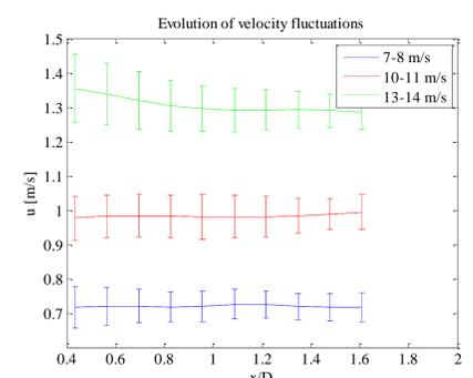
Fig. 4 Evolution of velocity fluctuations  $u'$  as a function of normalized axial distance for various free-stream velocities for  $0.09 \leq TI \leq 0.10$
