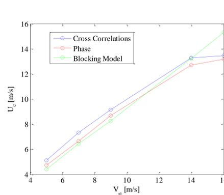
Fig. 5 Comparison of the various methods utilized to estimate the convective velocities  $U_c$
