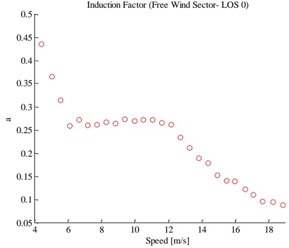
Fig. 4 Evolution of induction parameter "a" as a function of free-stream wind speed.
