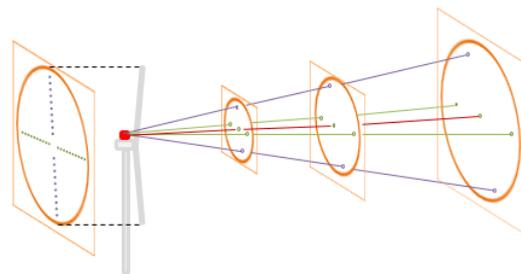
Fig. 2 LiDAR beam configuration.
