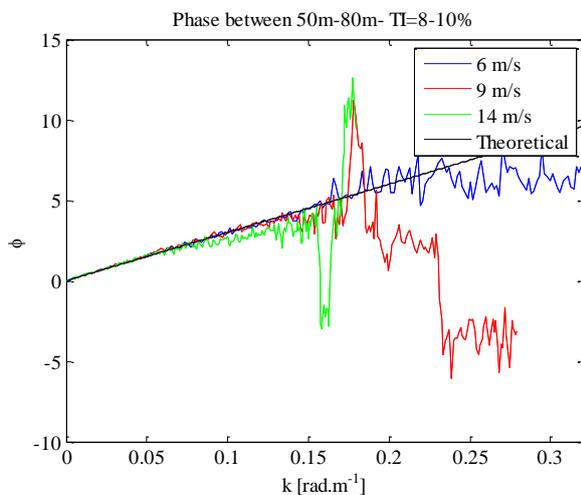
Fig. 9 Phase angle, in radians, of measurements taken at two upstream location for various free stream wind speeds, as a function of wavenumber  $k = 2\pi/Vt$ .
