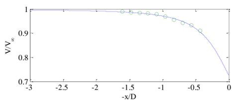
Fig. 1 Free-stream velocity as a function of the distance from the rotor (circles), together with fitted wind model to determine the induction parameter.
