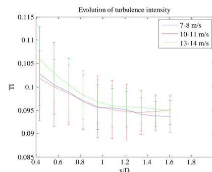
Fig. 3 Evolution of turbulence intensity as a function of normalized axial distance for various free-stream velocities for  $0.09 \leq TI \leq 0.10$
