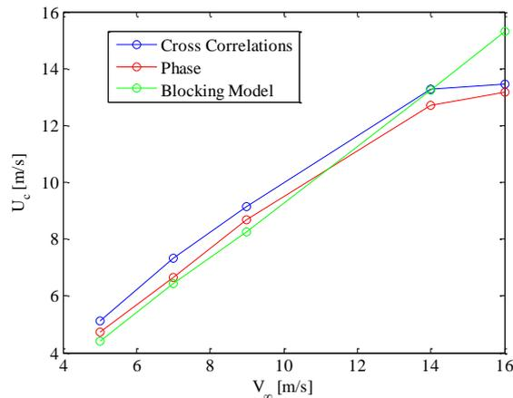
Fig. 8 Comparison of the various methods utilized to estimate the convective velocities  $U_c$ .
