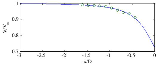
Fig. 3 Free-stream velocity as a function of the distance from the rotor (circles), together with fitted wind model to determine the induction parameter.
