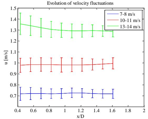
Fig. 7 Evolution of velocity fluctuations  $u'$  as a function of normalized axial distance for various free-stream velocities for  $0.09 \leq TI \leq 0.10$
