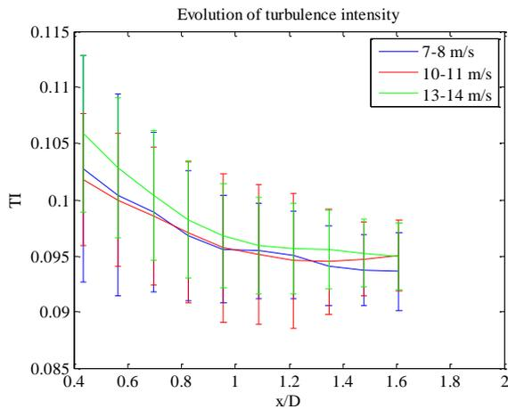
Fig. 6 Evolution of turbulence intensity as a function of normalized axial distance for various free-stream velocities for  $0.09 \leq TI \leq 0.10$ .
