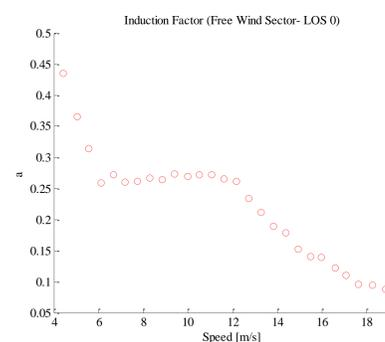
Fig. 2 Evolution of induction parameter "a" as a function of free-stream wind speed.
