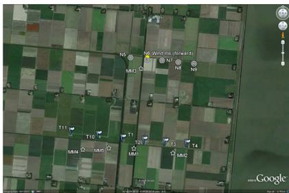
The North part of the site consists of 5 ECN research turbines in a row from East to West with a rated power of 2.5MW, a rotor diameter of 80m and a hub height of 80m. The second turbine from the East is the turbine under test. Directly South-West of this turbine at 2.5D a fully IEC compliant, 108m high meteorological mast (MM3) is located with boom measurements at hub height.
