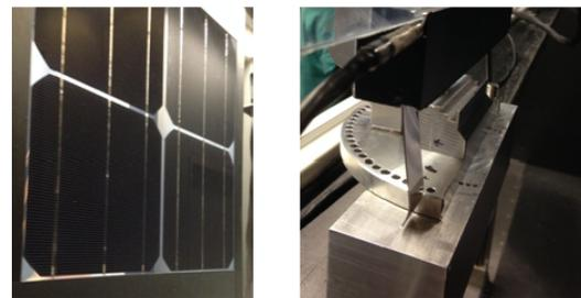
**Figure 2:** (left) Bifacial n-Pasha module, showing the masked aperture. (right) Angular dial used to rotate the module in the Pasan flash tester with 5° resolution.
