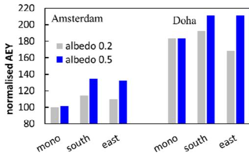
**Figure 8:** Normalised AEY for modules without LTF for the three model systems: *mono* = equator-facing monofacial module; *south* = same for bifacial module; *east* = vertical, east/west facing bifacial module. Equator-facing systems were evaluated at 38° tilt (Amsterdam, left) or 25° tilt (Doha, right)
