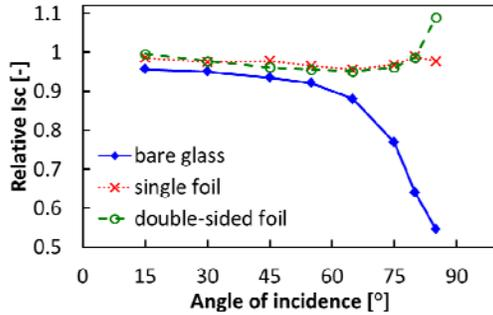
**Figure 6:** Relative Isc, i.e. Isc divided by  $\cos(\theta)$ , as a function of  $\theta$
