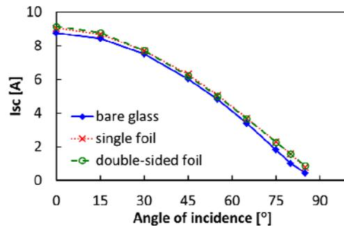
**Figure 5:** Short-circuit current  $I_{sc}$  as a function of the angle of incidence  $\theta$ . The data points for single foil and double-sided foil are almost overlapping
