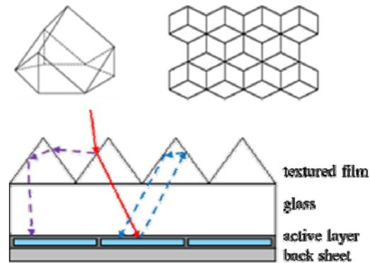
**Figure 1:** (top) Structure of light trapping film. (bottom) Schematic cross-section of PV module with LTF showing the working principle.
