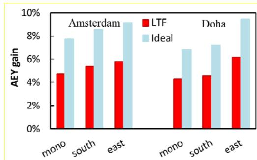
**Figure 9:** Same as Figure 8, but now showing the relative increase in AEY for each situation due to LTF (red) at low albedo. In light blue, the maximum gains are shown, corresponding to no reflective losses at any angle
