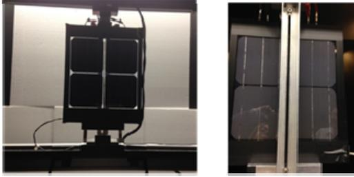
**Figure 3:** (left) Bifacial n-Pasha module in front of the “albedo” created by the Styrofoam panels. (right) Rear view of the angular dial showing that all cells are slightly shaded by the rotating beam
