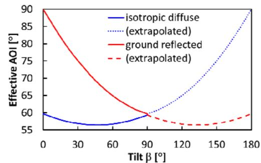
**Figure 7:** Effective angle of incidence as a function of tilt angle  $\beta$  for isotropic diffuse and ground reflected contributions to the incident light [2]. Dashed lines are approximations for the rear side (tilt larger than  $90^\circ$ )
