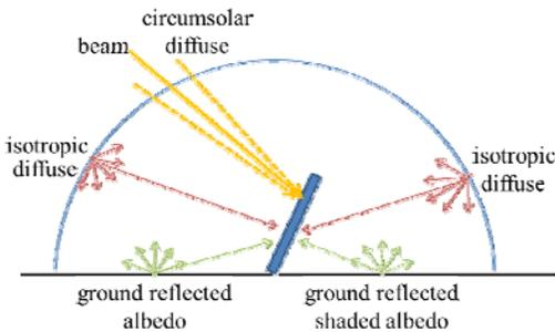
**Figure 4:** Overview of all the light components in the anisotropic sky model. After Duffie and Beckman [2]
