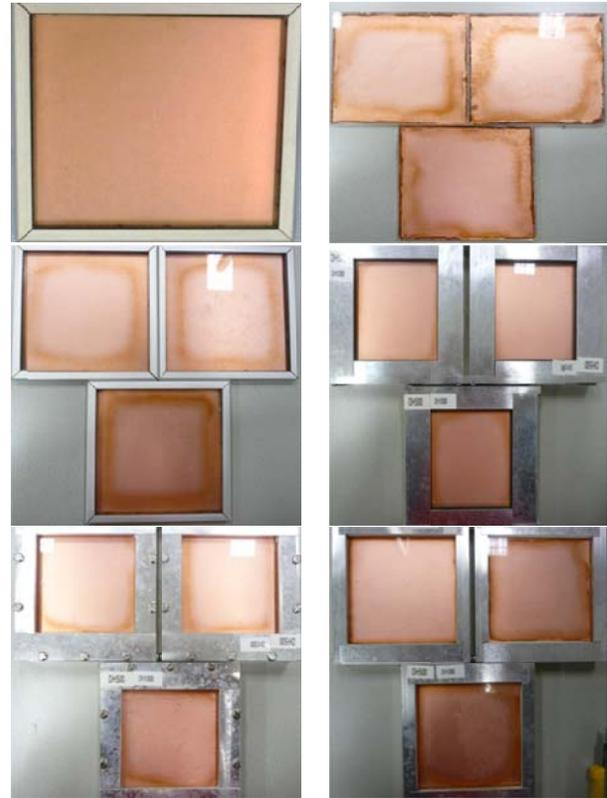
**Figure 4:** Visual appearance of tested coupons with alternative edge sealants after 1000 hours in DH. Upper left: sample before DH test. Upper right: without edge sealant. Middle right: double side adhesive tape (reference). Middle right: U-profile. Below left: “O”-ring and below right: sponge rubber
