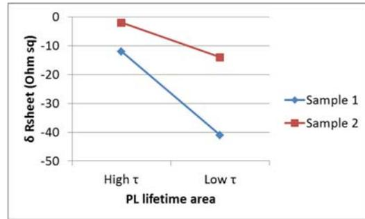
Figure 6: change in resistivity due to a forming gas anneal for high and low lifetime wafers. Samples originate from different ingots.
