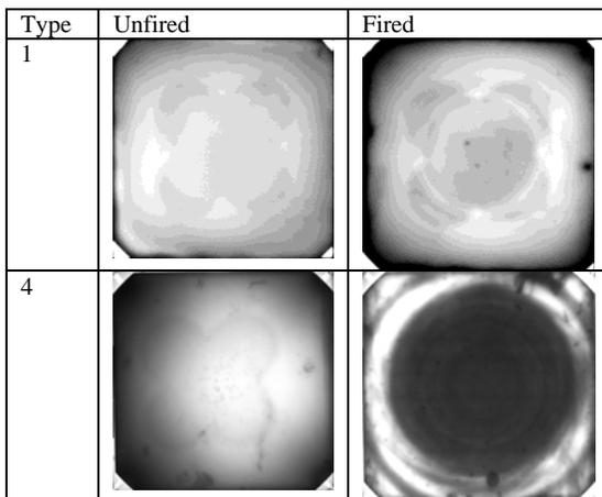
Figure 3: effect of firing on group 1 (SiN with emitter + BSF) or group 4 (SiN doped layers removed) for neighbouring wafers. The doped layers decrease the ring effect due to relatively low lifetimes in the doped layers.
