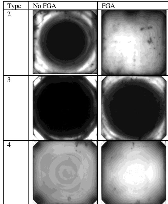
Figure 4: Effect of FGA performed before capping the samples for a-Si (2) AlOx(3) and SiN (4) capped samples. The SiN samples are unfired as firing negates the differences between the samples.
