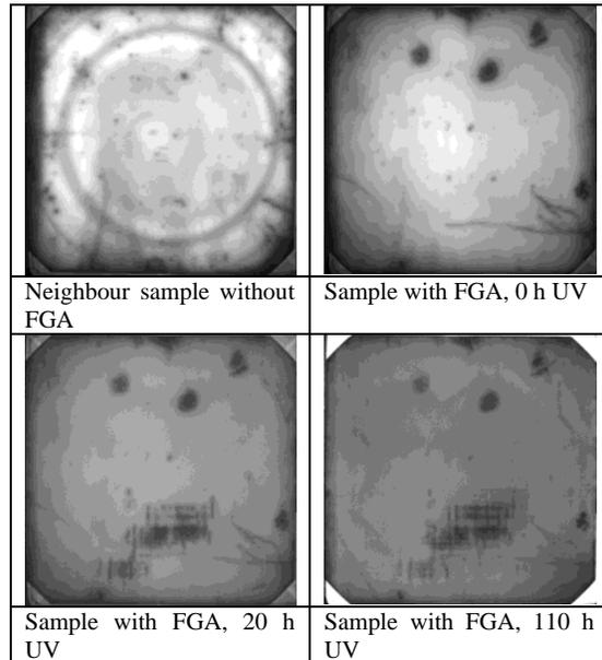
Figure 7: PL images for a sample without FGA compared to a sample with FGA which is subjected to UV weathering.
