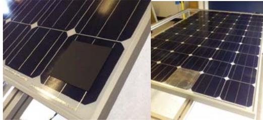
Figure 1: Impression of the opaque and wire meshes used for the shading correlation experiments under a steady state solar simulator
