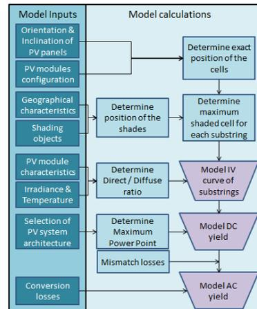
Figure 6: Yield model inputs and flow of simulation processes
