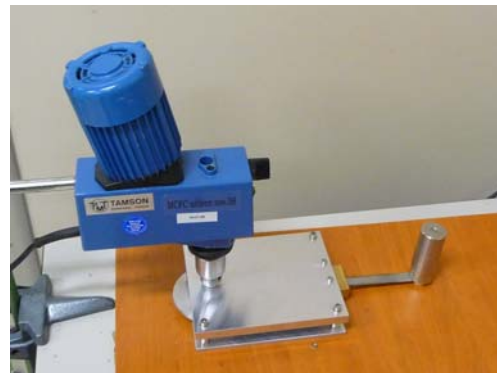
Figure 1: Felt rubbing test setup
