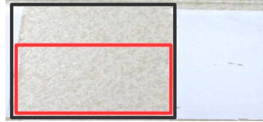
Figure 3: A glass sample (no. 3) with anti-soiling coating after abrasion testing (> 10000 strokes), soiling (white material) and removal of loosely adhered soiling material
