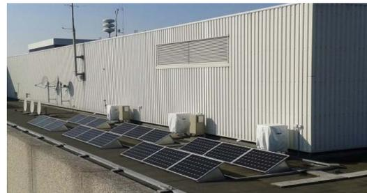
**Figure 3 :** Impression of the field test. Every PV system consists of two successive rows of three solar panels. On the right side is the micro inverter system while in the middle is the reference string inverter system. On the far left is the power optimizer system. The measuring equipment and inverters are located in the cabinets behind the panels.
