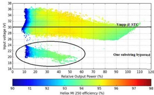
**Figure 7:** Relation of input voltage with efficiency and power output during 5 months of operation under clear and partially shaded conditions. The micro inverter includes a hybrid P&O MPPT algorithm which can track global maximum by performing regularly IV scans.
