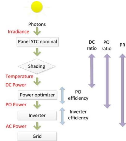
**Figure 5.** Schematic rep of the path from sunlight into grid injected AC power, showing the monitored parameters in red and the definition of the DC ratio, PO ratio and PR on the right hand side by blue and purple arrows
