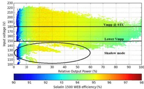
**Figure 6:** Relation of input voltage with efficiency and power output during 5 months of operation under clear and partially shaded conditions. Note that the input voltage is reduced significantly during shade mode operation under partially shaded conditions.
