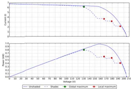
**Figure 2:** Measured IV and PV curve of an unshaded and partially shaded PV system with a pole. In this case three local maxima and a global maximum peak can be observed. Traditional MPPT techniques have difficulties tracking the dynamics of partially shaded series connected PV modules.
