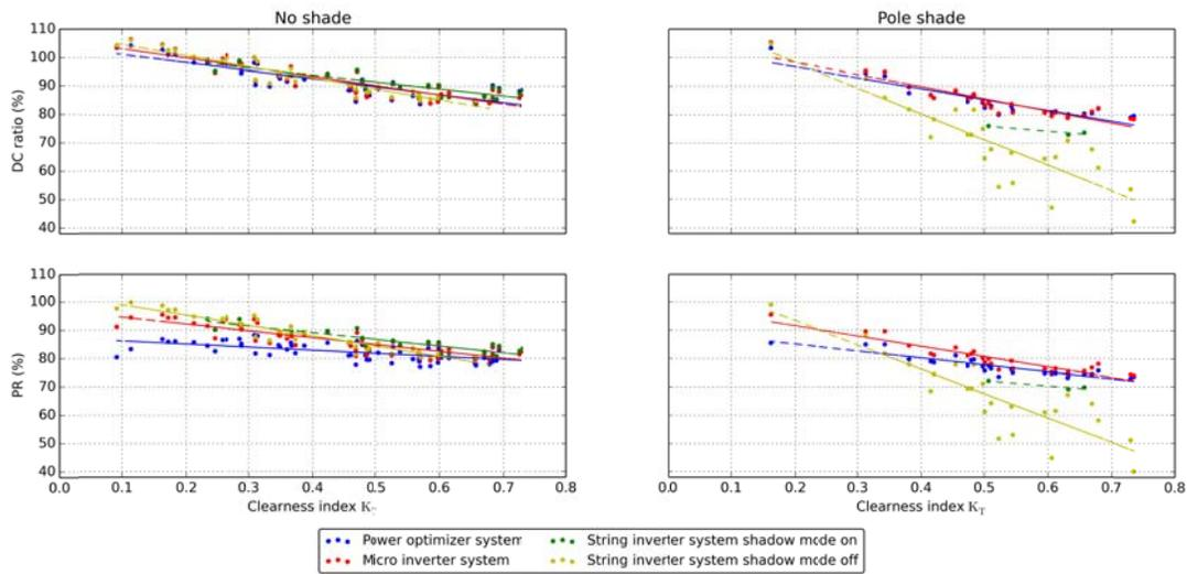
**Figure 9:** Daily calculated PR and DC ratio versus average clearness index of the day for unshaded and partially shaded operation of the three systems with a pole shading 1-2% of the total PV system surface. Data presented at the graph are calculated during spring months.
