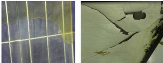
**Figure 4:** Images showing module B tested above 85°C. The left image shows melted encapsulant on the front of the module glass. The right image shows the rear of the module with the back-sheet fractured by the movement of the encapsulant and encapsulant on the outside of the back-sheet
