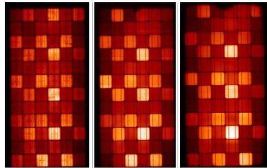
**Figure 6:** EL images of module C following degradation during damp-heat testing. The left image shown the start condition of the module, the centre image the condition after 2000 hours at 95°C and 85%RH and the right image the condition after 3000 hours. A limited amount of degradation can be seen after 3000 hours with dark areas at the edge of the module and at the location of the junction box
