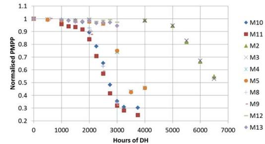
**Figure 1:** Plot of degradation in damp-heat for module A. The legend correspond to the test codes in table 2
