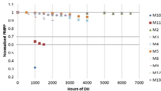
**Figure 3:** Plot of degradation in damp-heat for module B. The legend corresponds to the test codes in table 2. The module is stable for temperatures at and below 85°C. Above this temperature the module fails catastrophically
