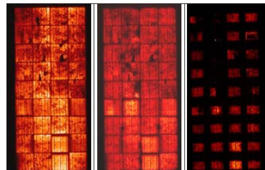
**Figure 2:** EL images of module A following degradation during damp-heat testing. The left image shown the start condition of the module, the centre image the condition after 2000 hours at 95°C and 85%RH and the right image the condition after 3000 hours. Moisture ingress results in degradation of the metallisation on the cell at the cell
