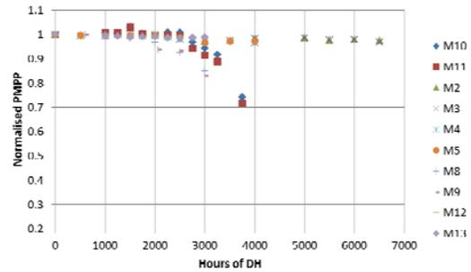
**Figure 5:** Plot of degradation in damp-heat for module C. The legend corresponds to the test codes in table 2. The module are very stable with degradation at the highest temperatures only seen after 2000 hours
