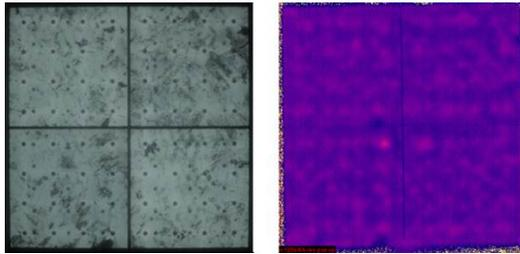
**Figure 4:** Left, EL image and, right, DLIT image of a four-cell module made with 100  $\mu\text{m}$  thick encapsulant with a reduced volume of conductive adhesive. The images are uniform in colour and similar to images obtained from module made with 200  $\mu\text{m}$  encapsulant and standard volume conductive adhesive contacts
