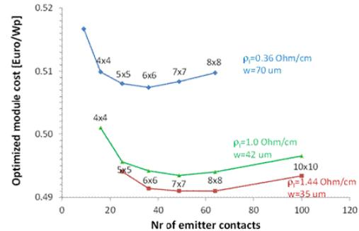
**Figure 6:** Optimised module cost for MWT cells with an increasing number of vias with different finger widths and line resistances. The reduced adhesive volume is included in these calculations. A cost reduction of close to 4% is predicted by going to a 6x6 or 7x7 via configuration in combination with a reduced finger width
