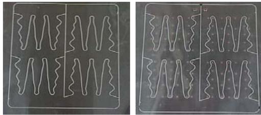
**Figure 2:** Left, an aluminium based conductive back-sheet patterned for a 4 cell module and right, the same foil with copper contacts applied by cold-spraying
