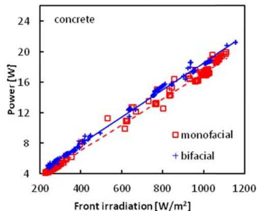
**Figure 6:** Maximum power as a function of front irradiation for a monofacial and a bifacial 2x2 mini-module at 38° tilt, south facing installation. The underground is concrete
