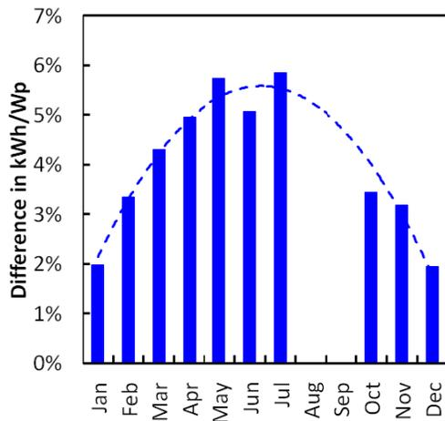
**Figure 4:** Difference between the bifacial and monofacial kWh/W<sub>p</sub> over the year, normalised to the monofacial kWh/W<sub>p</sub>
