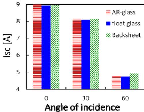
**Figure 1:**  $I_{sc}$  of bifacial modules as a function of the angle of incidence with three different back sheet materials
