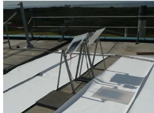
**Figure 5:** Photograph of the set-up showing the monofacial and bifacial mini-modules with the white underground. Note the less dark shadow of the bifacial module due to its transparency.
