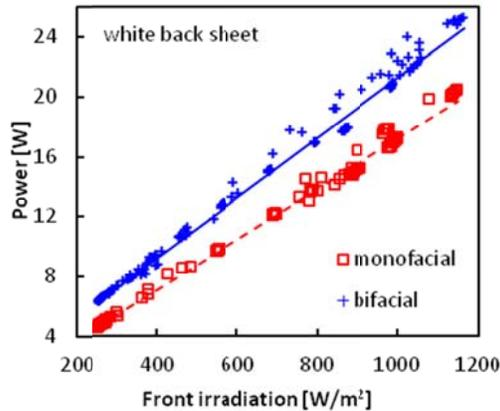
**Figure 7:** Maximum power as a function of front irradiance for a monofacial and a bifacial 2x2 mini-module at 38° tilt, south facing installation. The underground is 4x4 m<sup>2</sup> white back sheet
