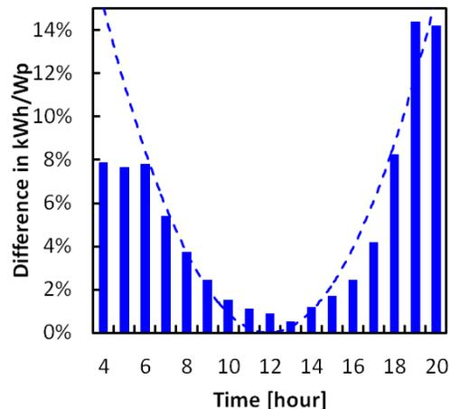
**Figure 3:** Normalised difference of the bifacial and the monofacial kWh/ $W_p$ , as a function of the time of day. The summed energy production in kWh is taken over the whole year
