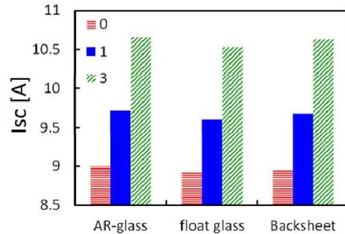
**Figure 2:**  $I_{sc}$  of bifacial modules with three different back sheet materials measured with various albedo, created by placing Styrofoam panels against the rear wall of the IV-flash chamber
