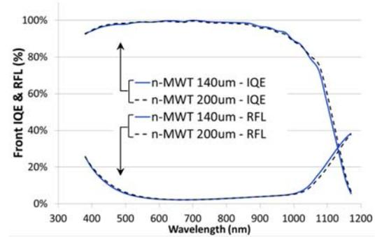
**Figure 7:** Internal quantum efficiency and Reflectance measured from the front side of n-MWT cells processed from 200  $\mu\text{m}$  and 140  $\mu\text{m}$  wafer thickness.
