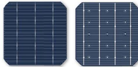
**Figure 2:** Image of an n-type MWT silicon solar cells ( $239\text{cm}^2$ ) with a H-pattern based unit cell design and 15 vias: front side (left picture) and rear side (right picture)
