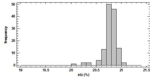
**Figure 6:** Efficiency distribution of 134 n-MWT cells fabricated with the optimized 6x6 via pattern and including recent n-Pasha improvements (before spectral mismatch correction).
