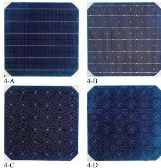
**Figure 4:** **A)** Front side 'new' nMWT: 6x6 vias with thin busbars. Metal fraction  $\sim 3.1\%$  of total cell area **B)** Rear side 'new' n-MWT: 6x6 emitter contacts and (7x7)-4 base contacts (corners are excluded due to the semisquare wafer **C)** Star pattern, metal fraction  $\sim 4.7\%$  of total cell area **D)** Circle pattern, metal fraction  $\sim 4.4\%$  of total cell area
