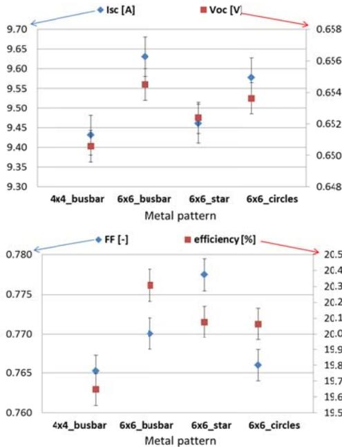
**Figure 5:**  $I_{sc}$ ,  $V_{oc}$  (top graph) and FF, Efficiency (bottom graph) of n-MWT cells with different amount of vias (16 and 36) and different front metal patterns.
