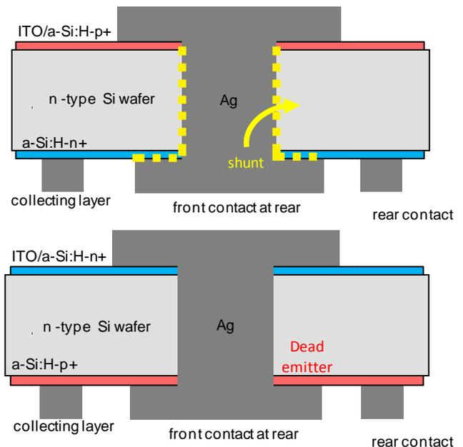
Figure 2. Structure of a front (top) and rear (bottom) emitter MWT-HJ solar cell.
