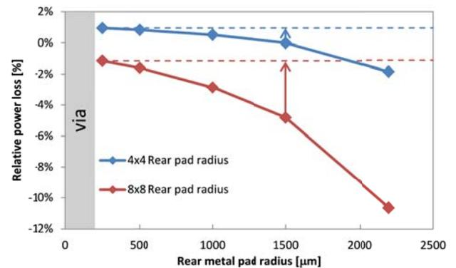
Figure 6. Calculated relative power losses for a 4x4 and 8x8 configuration as function of the rear pad radius (front metal contact at the rear). The arrows represent an estimate of the gain when isolating the real metal pad, equivalent to the smallest rear metal pad radius, and the dashed lines are a guide for the eye. Dead emitter area per via is kept constant. In the experiment reported in this paper we used a 4x4 configuration with a rear metal pad radius of 1.5mm (reference).
