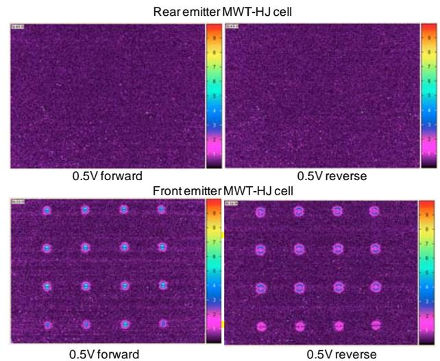
Figure 4. Lock In Thermography of a *front emitter* and *rear emitter* solar cell in forward and reverse currents. The advantage of the *rear emitter* configuration with respect to the absence of shunts at the vias is clear.
