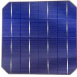
Figure 1. Image of the MWT-HeteroJunction solar cell as presented in this paper.
