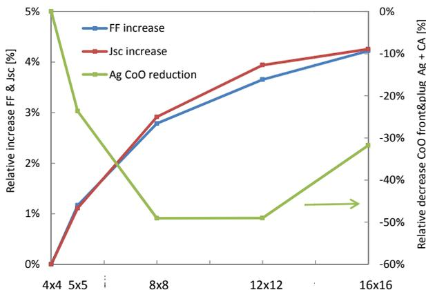
Figure 5. Calculated relative FF and Jsc variations as a function of the number of vias for MWT-HJ cells. The cost of ownership (CoO) reduction of the front contact silver including plug and conductive adhesive (CA) is also calculated (right axis).
