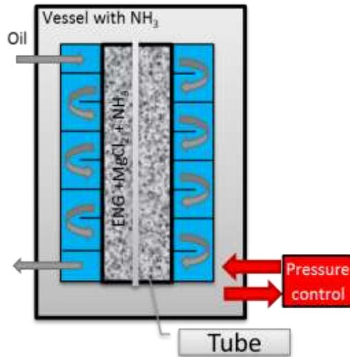
Figure 5: Schematic view of experimental setup
