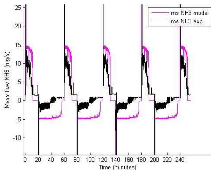
Figure 8: The measured (black) and calculated (pink) mass flow of  $\text{NH}_3$  as a function of time.
