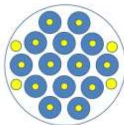
**Figure 3: Schematic representation of lab scale shell-n-tube type reactor with blue the sorbent material and in yellow the open gas volume – allowing the sorbate to flow through the tubes and the white represents the heat transferring medium.**
