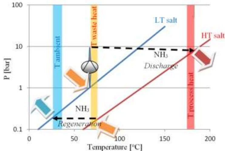
Figure 2: Schematic representation of the cycle of the hybrid heat pump type II configuration
