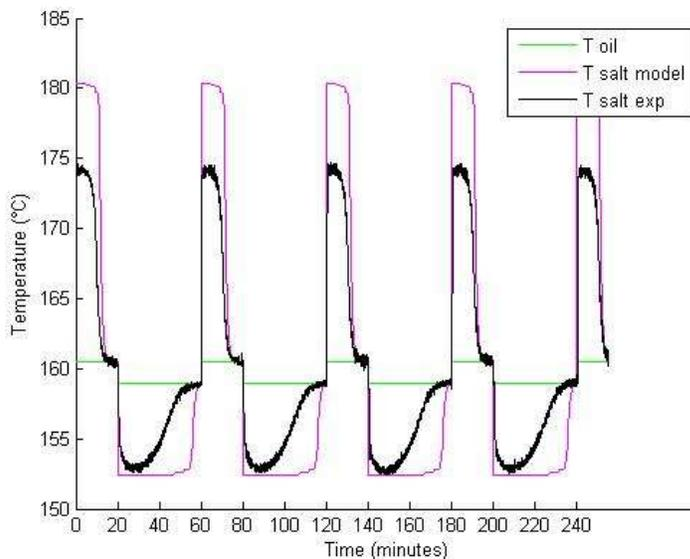
**Figure 7: The relation between temperature of thermal oil (measured = green) and salt (measured = black, calculated = pink) as a function of time.**
