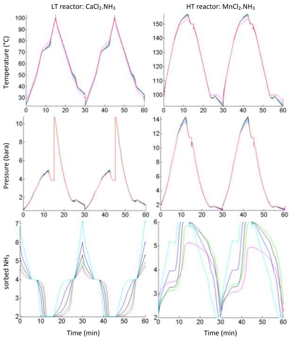
Figure 6: Model calculations of sorbent temperature, pressure and amount of  $\text{NH}_3$  sorbed as a function of time for a system with 1 MW heat output
