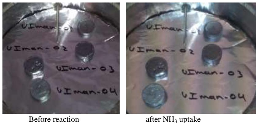
**Figure 4:** Overview of composites before and after reaction with NH<sub>3</sub>
