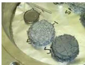
**Figure 3:** Picture of the composite obtained in dry mixing procedure, after reaction with NH<sub>3</sub>. Top left pellet is graphite without salt.
