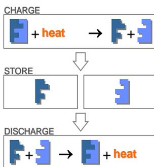
Figure 1: Concept of thermochemical heat storage.
