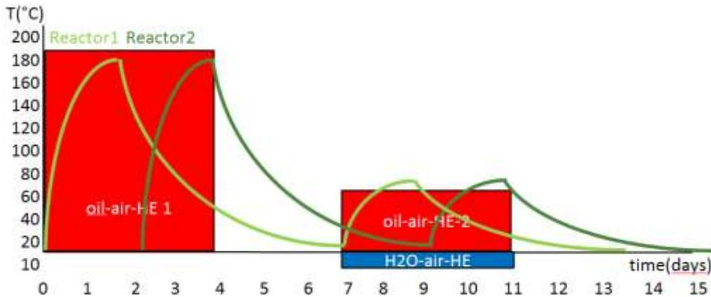
Figure 4: Simplified temperature profiles for the zeolite reactors during the charge and discharge measurement. The green lines indicate the evolution of the reactor temperatures
