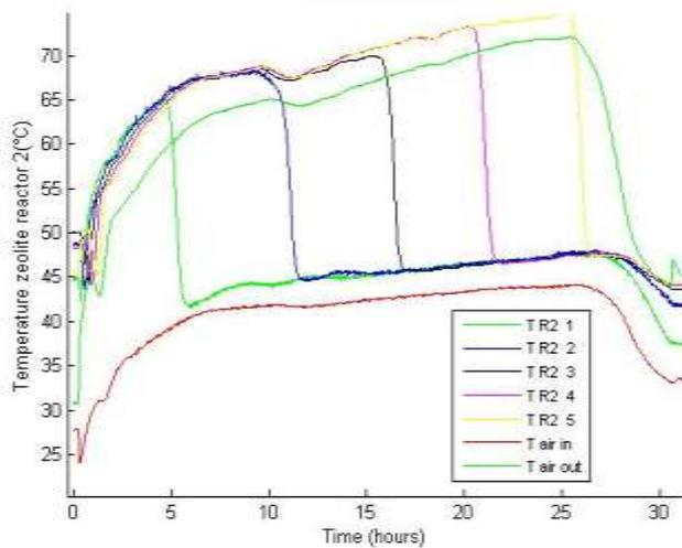
Figure 6: Temperature over time of the air and the zeolite bed of reactor 2 during the discharge process
