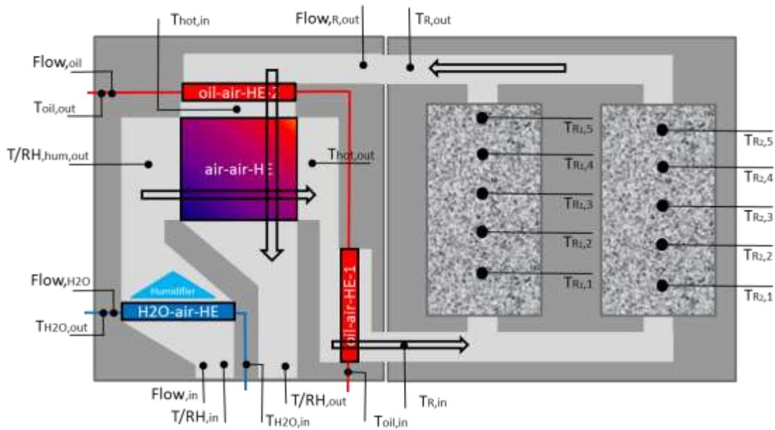
Figure 2: Process flow diagram and instrumentation for the open sorption prototype system.
