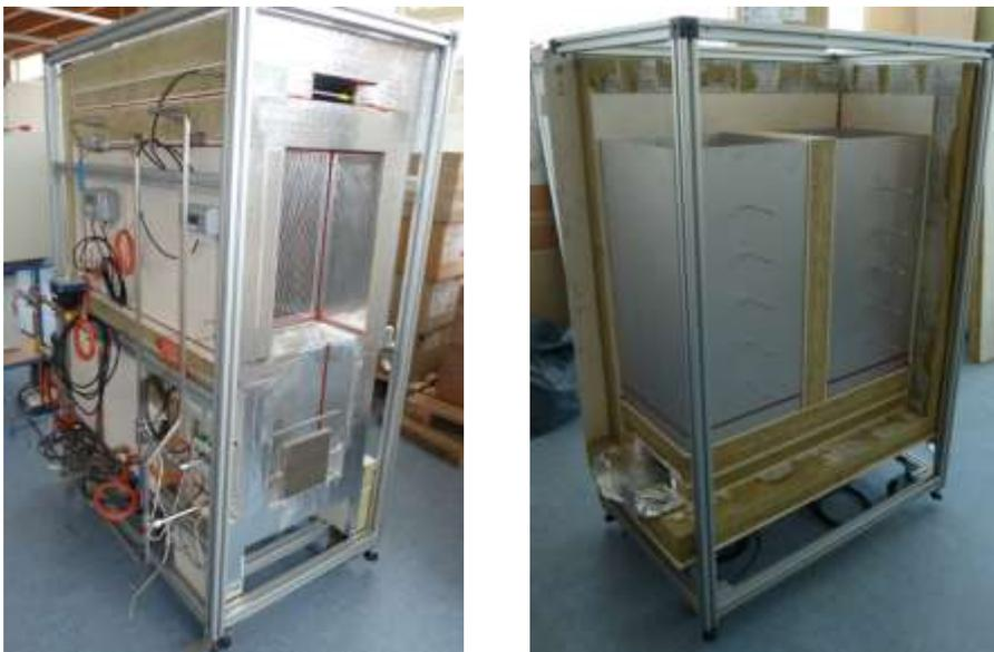
Figure 3: Pictures of the open sorption prototype system under construction. Left: the air handling section, right: the storage containers section
