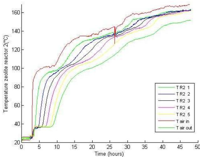
Figure 5: Temperature over time of the air and the zeolite bed of reactor 2 during charge process
