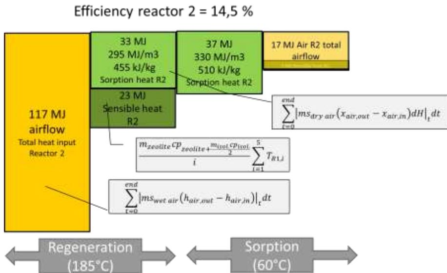
Figure 7 Analysis of the overall storage cycle efficiency for reactor 2.
