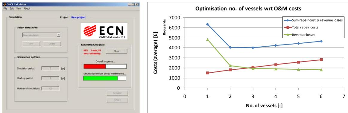
Figure 4: The OMCE-Calculator: ECN's software for advanced OPEX cost modelling. On the left an example of its GUI, on the right an example to find the optimal number of access vessels.
