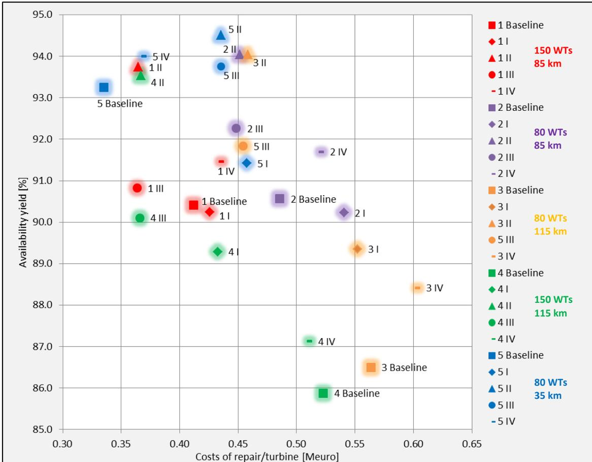
Figure 6: Key simulation results for the five considered O&M concepts for each of the five modelled offshore wind farms.
