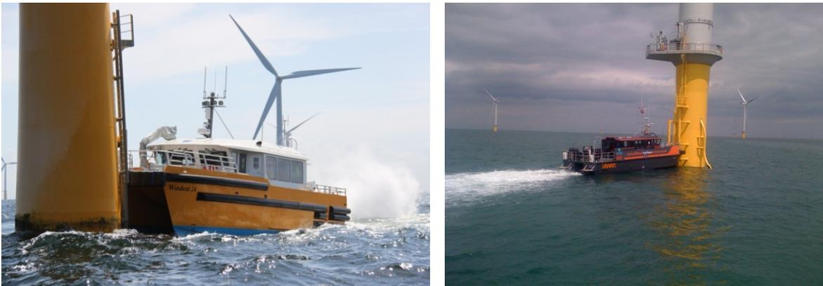
Figure 2: Examples of catamaran-like workboat access vessels: the WindCat MKIII on the left [2] and the CTruk 20T on the right [3].
