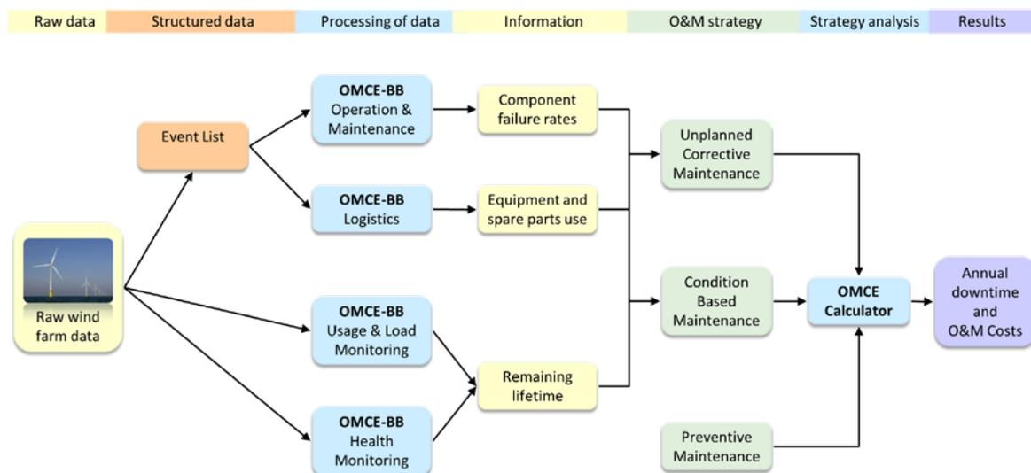
Figure 1-1: Structure of OMCE showing the steps from structuring operational data in the Event List format through data processing with the OMCE Building Blocks and modelling O&M strategies and performing analyses with the OMCE-Calculator.
