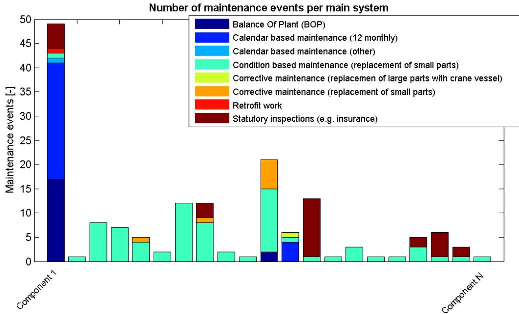
Figure 3-1: Examples of BB O&M ranking analyses results: overview of number and type of maintenance events per component
